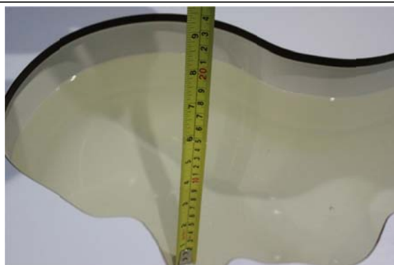
Liquid depth in the head phantom (2600MHz)
