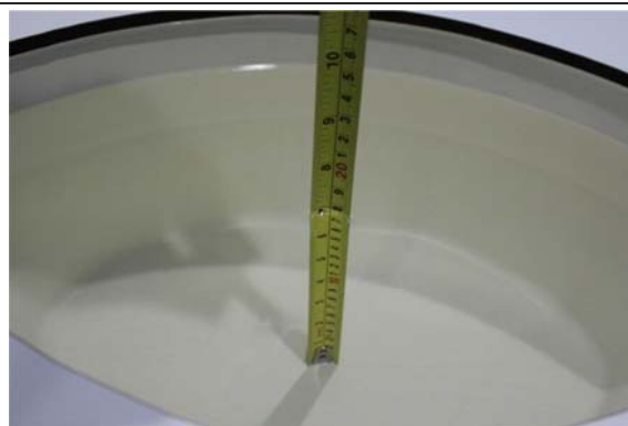
Liquid depth in the body phantom (2600MHz)
