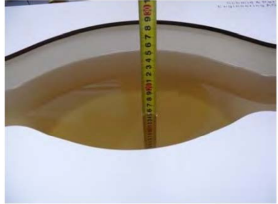
Liquid depth in the body phantom (835MHz)
