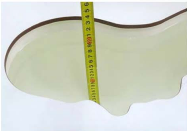
Liquid depth in the head phantom (1900MHz)
