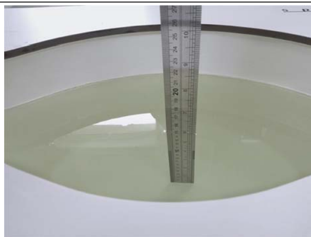
Liquid depth in the body phantom (2450MHz)
