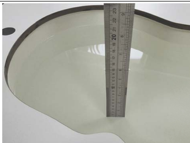
Liquid depth in the head phantom (2450MHz)
