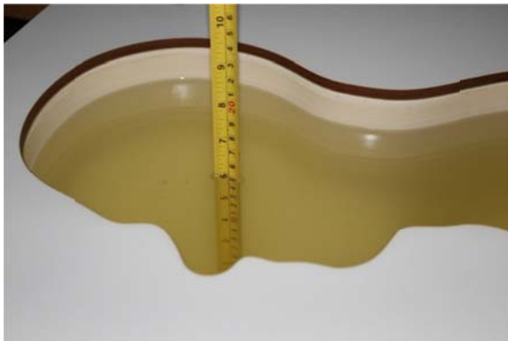
Liquid depth in the head phantom (1750MHz)
