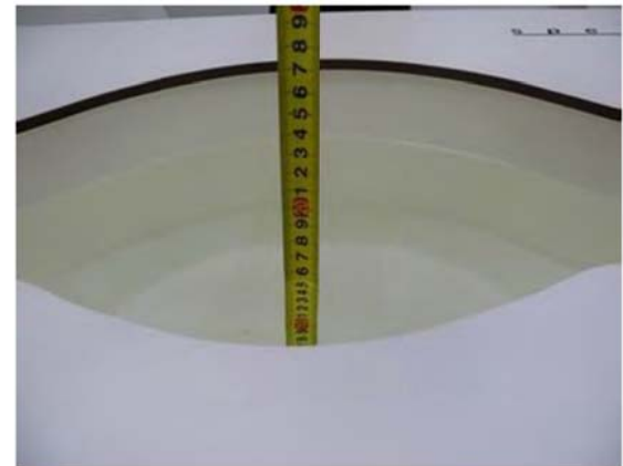
Liquid depth in the body phantom (1900MHz)
