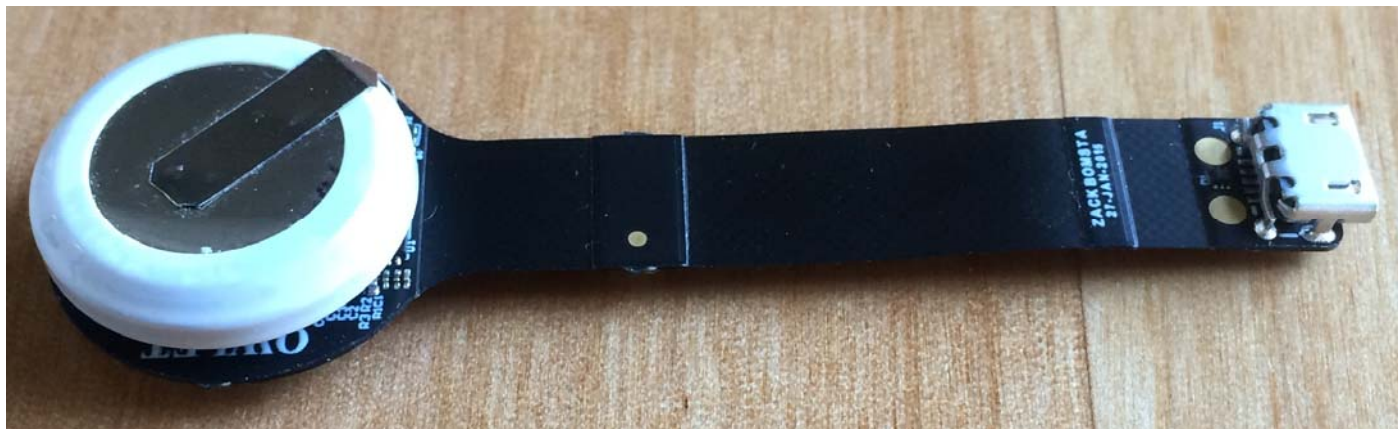
Figure 1 - Owlet Wearable Sensor - Showing Battery & Battery Clip
