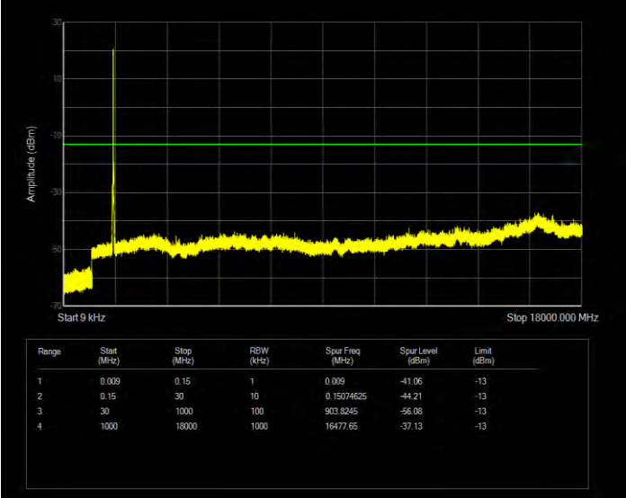
Band66 QPSK BW=10MHz Channel=132322 RB Size=50 Position=#0
