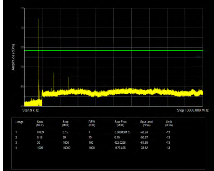
Band5 16QAM BW=1.4MHz Channel=20643 RB Size=6 Position=#0
