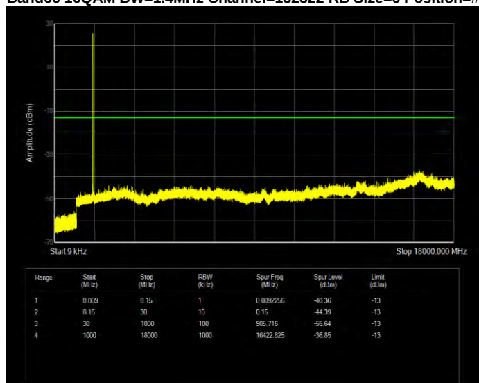
Band66 16QAM BW=1.4MHz Channel=132322 RB Size=6 Position=#0
