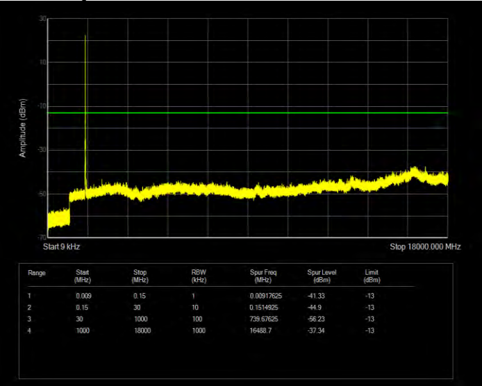
Band66 16QAM BW=5MHz Channel=132322 RB Size=25 Position=#0
