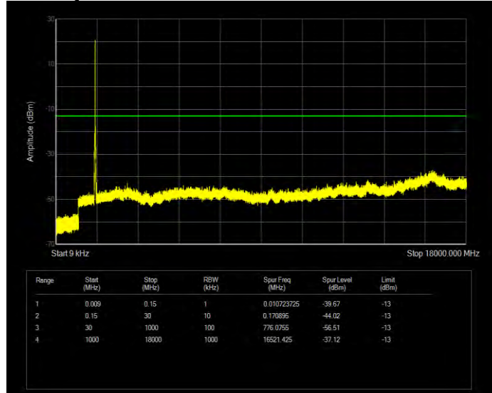
Band4 QPSK BW=10MHz Channel=20350 RB Size=50 Position=#0
