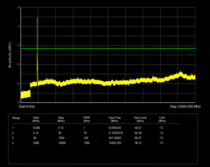
Band66 QPSK BW=15MHz Channel=132322 RB Size=75 Position=#0
