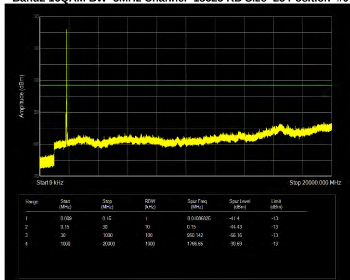
Band2 16QAM BW=5MHz Channel=18900 RB Size=25 Position=#0
