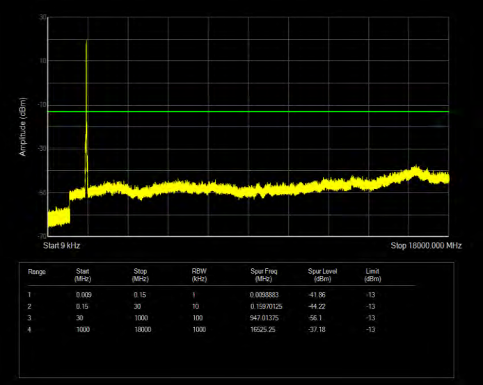
Band66 QPSK BW=20MHz Channel=132322 RB Size=100 Position=#0
