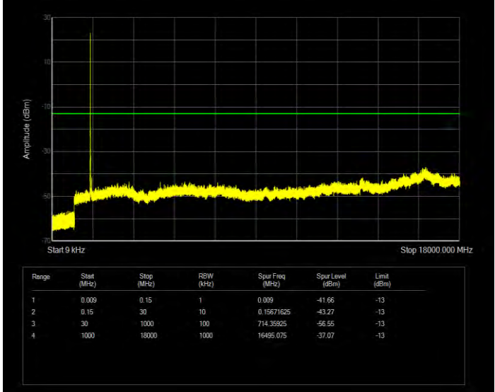
Band66 QPSK BW=3MHz Channel=132322 RB Size=15 Position=#0
