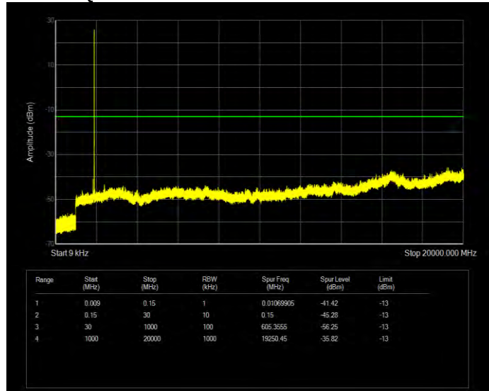
Band2 16QAM BW=1.4MHz Channel=19193 RB Size=6 Position=#0
