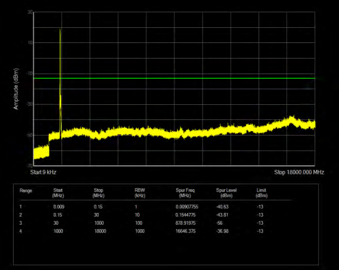
Band66 QPSK BW=20MHz Channel=132322 RB Size=100 Position=#0
