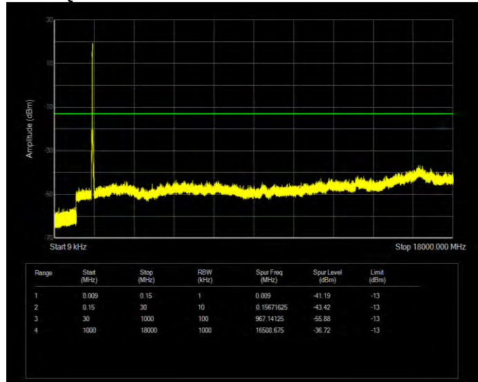
Band4 QPSK BW=20MHz Channel=20300 RB Size=100 Position=#0
