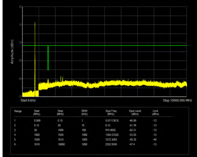
Band17 16QAM BW=5MHz Channel=23755 RB Size=25 Position=#0
