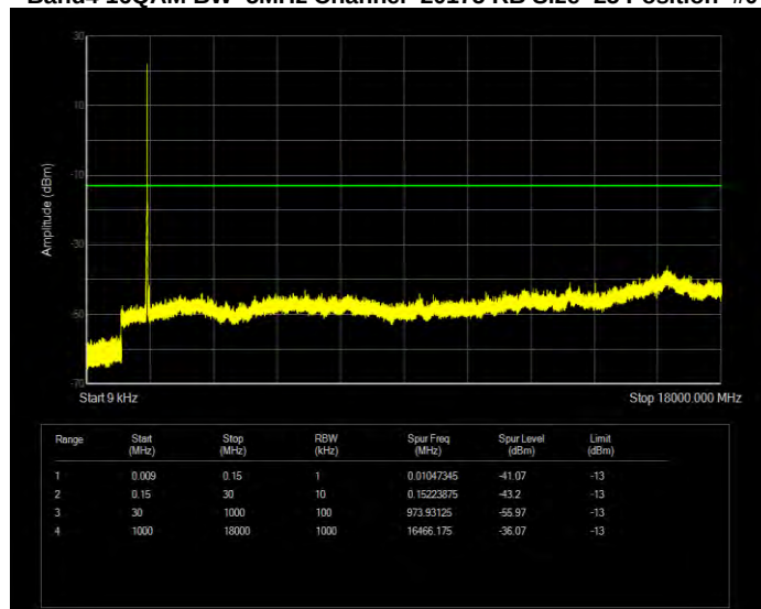
Band4 16QAM BW=5MHz Channel=20375 RB Size=25 Position=#0
