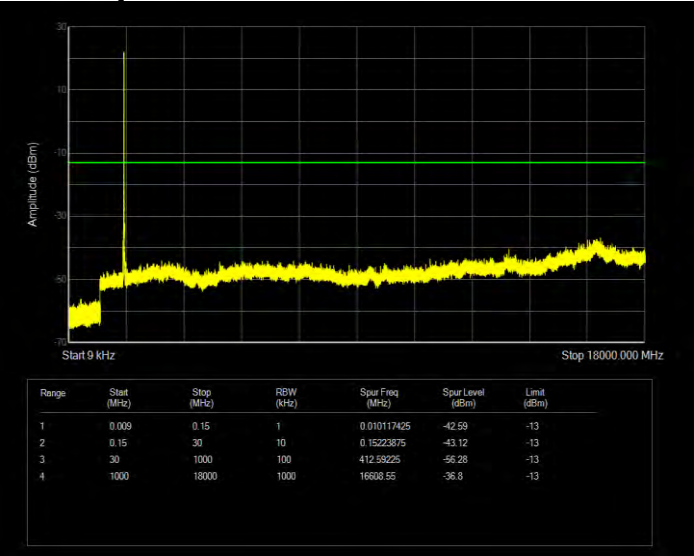
Band66 16QAM BW=5MHz Channel=132322 RB Size=25 Position=#0
