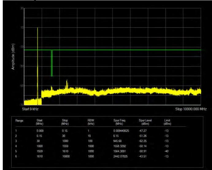
Band13 QPSK BW=5MHz Channel=23205 RB Size=25 Position=#0
