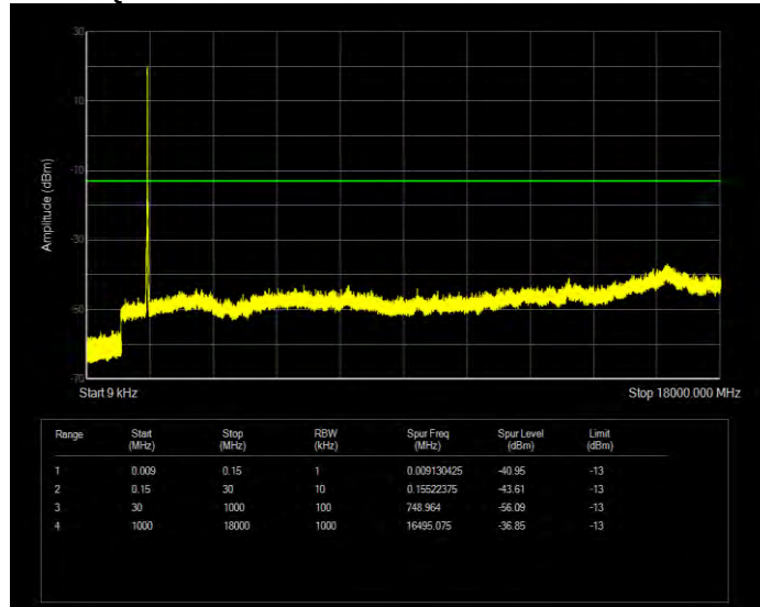
Band4 QPSK BW=10MHz Channel=20350 RB Size=50 Position=#0
