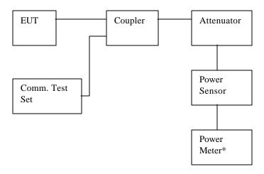
(\*) Power meter, spectrum analyzer & CMU 200 Communication Tester were used.
