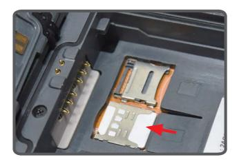
**Insert SIM Card:** Insert the SIM card in the direction shown.
