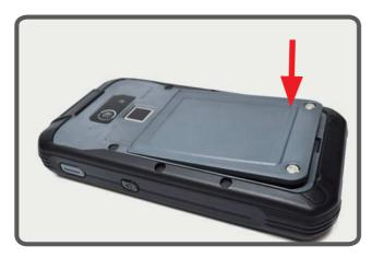
**Step 3:** Use the flathead screwdriver to tighten the two screws to ensure the waterproof performance.
