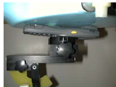
Figure 18. Hand SAR Test Setup
