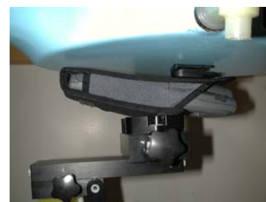
Figure 17. Body SAR Test Setup w/Holster
