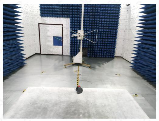
RADIATED EMISSION TEST SETUP ABOVE 1GHz
