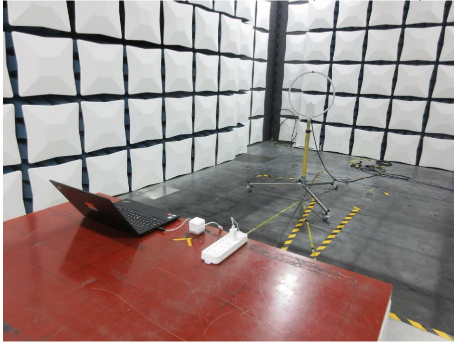
RADIATED RF MEASUREMENT SETUP (9KHz ~ 30 MHz)
