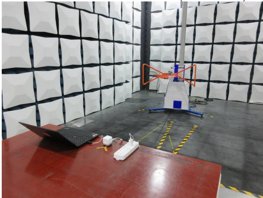
RADIATED RF MEASUREMENT SETUP (30MHz ~ 1 GHz)
