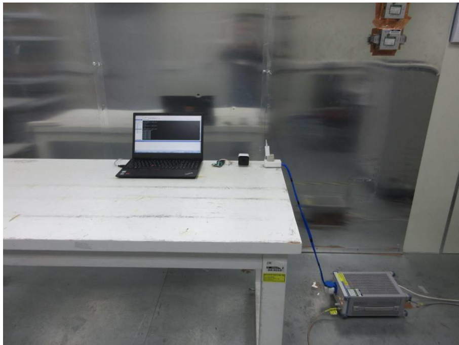
POWERLINE CONDUCTED EMISSIONS MEASUREMENT SETUP
