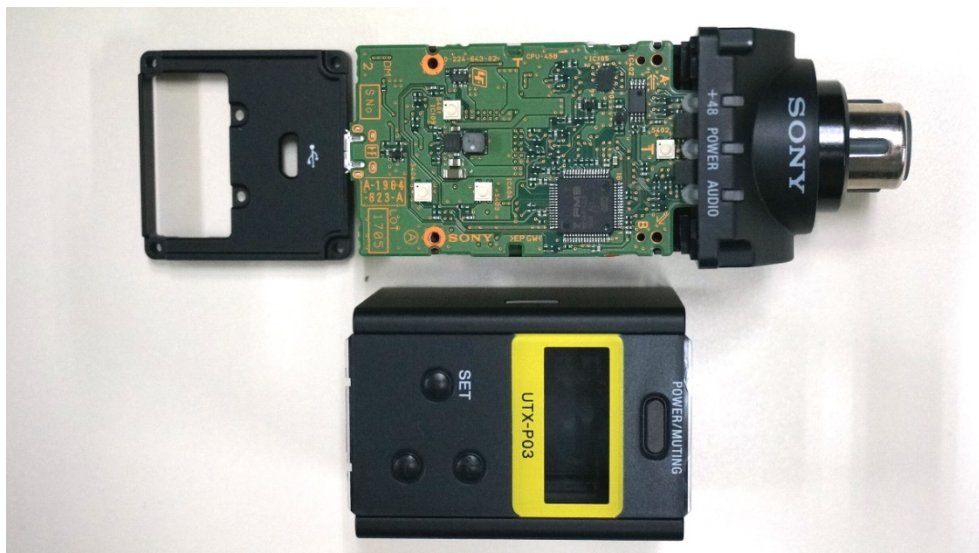
Fig.1: Removed the Case (Place of board CPU-458)
