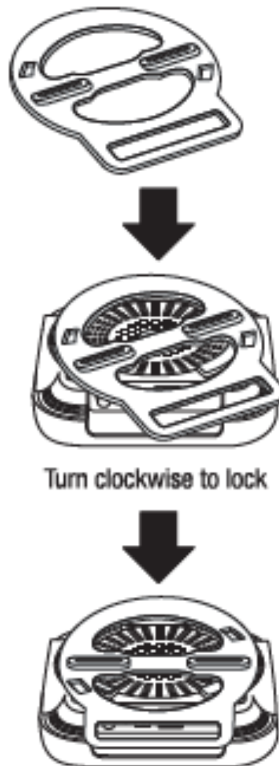
Figure 4: Locking the AP300 to Mounting
