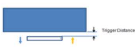
Picture : Proximity sensor triggering distances assessment (Back side)
