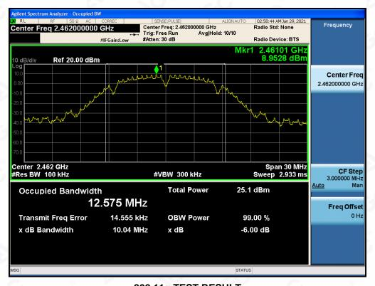
**802.11g TEST RESULT**TEST PLOT OF BANDWIDTH FOR LOW CHANNEL
