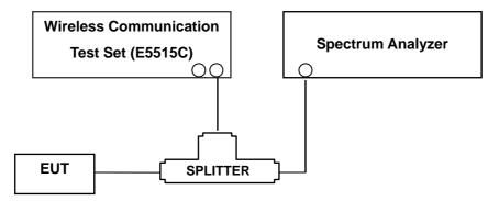
(Configuration of conducted Emission measurement)
