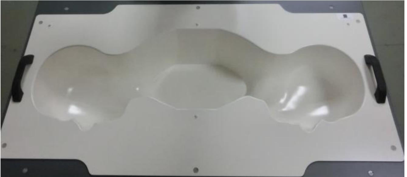
The SAM phantom is used to measure the SAR relative to people exposed to electro-magnetic field radiated by mobile phones.
