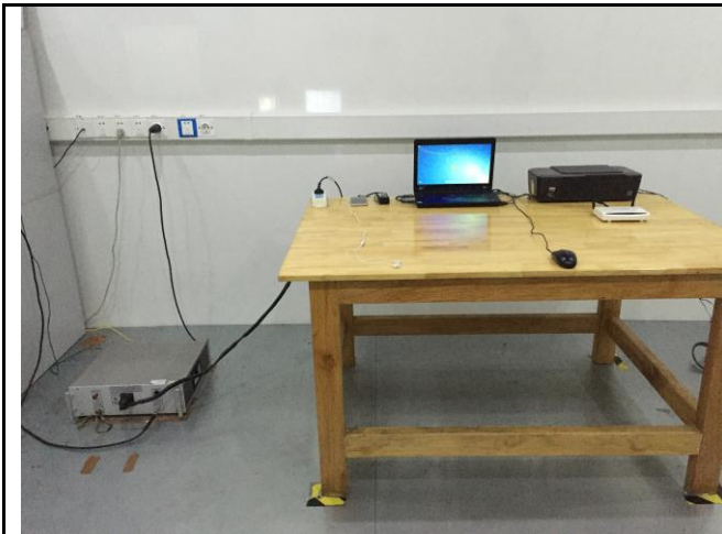
Conducted Emissions Test Setup – Front View
