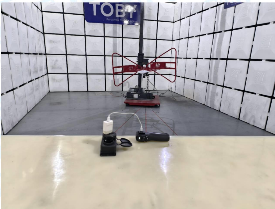
Photo of Setup for Radiated Emission (30MHz~1GHz)
