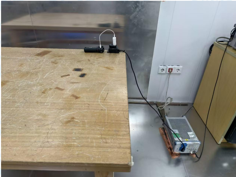
Photo of Setup for Radiated Emission (30MHz~1GHz)
