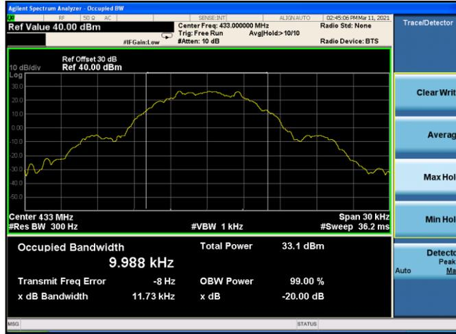
**GMSK 25KHz Channel Spacing: Occupied Bandwidth**
