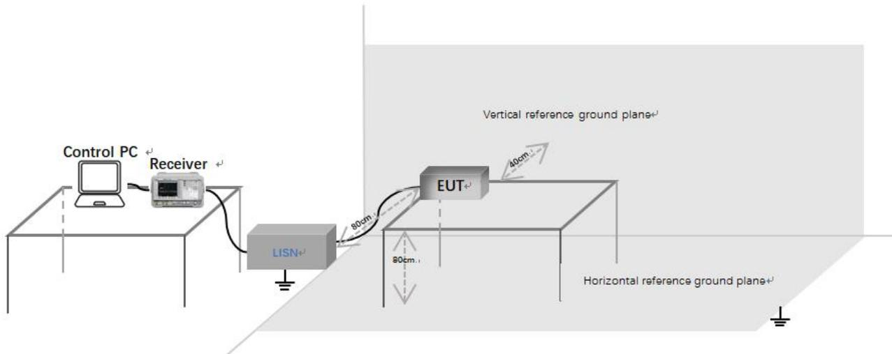
Description of test setup connection:
