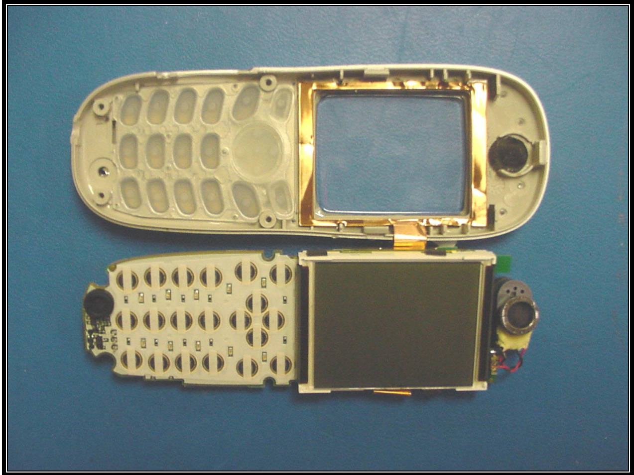
PHOTOGRAPH 18: PCB FRONT WITH LCD
