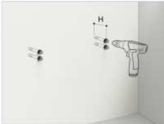
• Drill at the four sites using a percussion drill and embed 4\times\varnothing 8 plastic expansion pipes.
