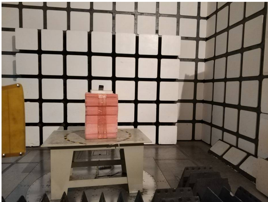
Radiated Emissions View (Above 1 GHz)
