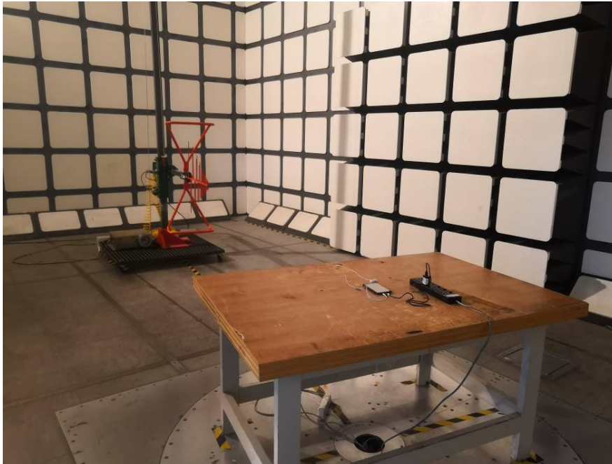
Radiated Emissions View (Below 1 GHz)
