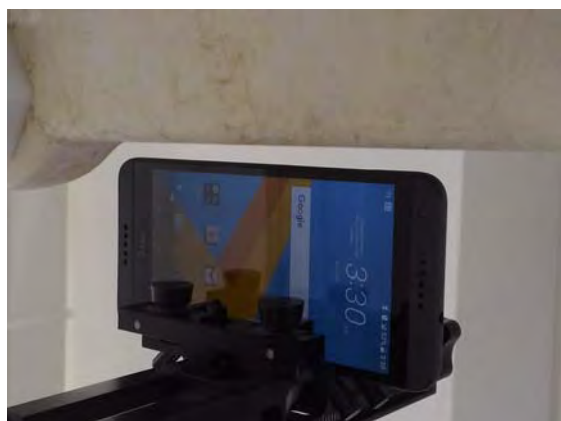
Fig.13 EUT Left side to flat phantom
