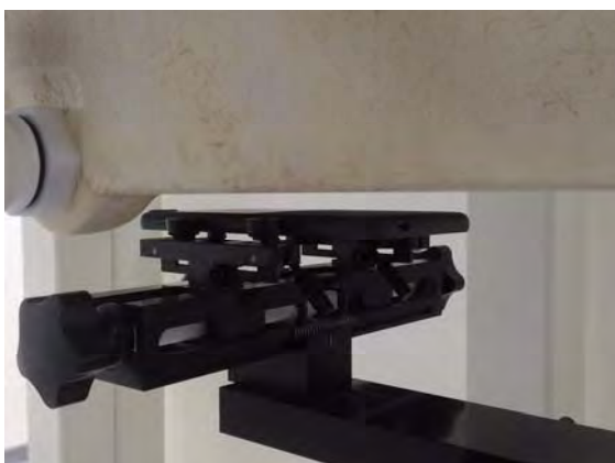
Fig.8 EUT Back side to flat phantom
