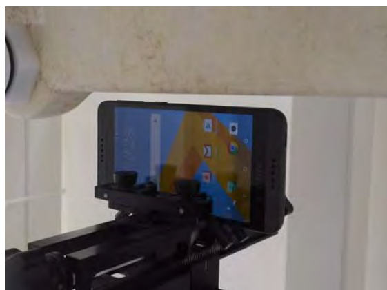
Fig.14 EUT Right side to flat phantom
