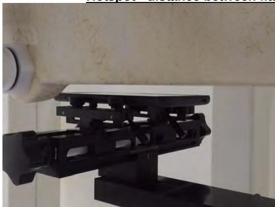
Fig.9 EUT Front side to flat phantom
