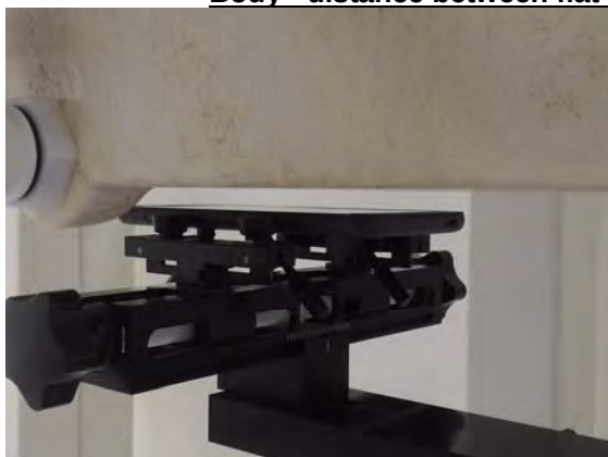
Fig.7 EUT Front side to flat phantom
