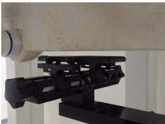
Fig.11 EUT Back side to flat phantom
