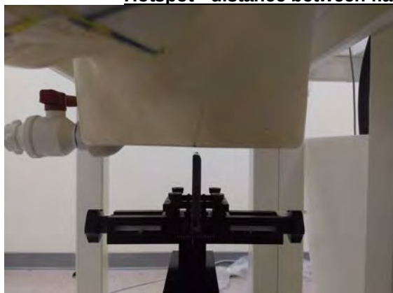
Fig.12 EUT Top side to flat phantom
