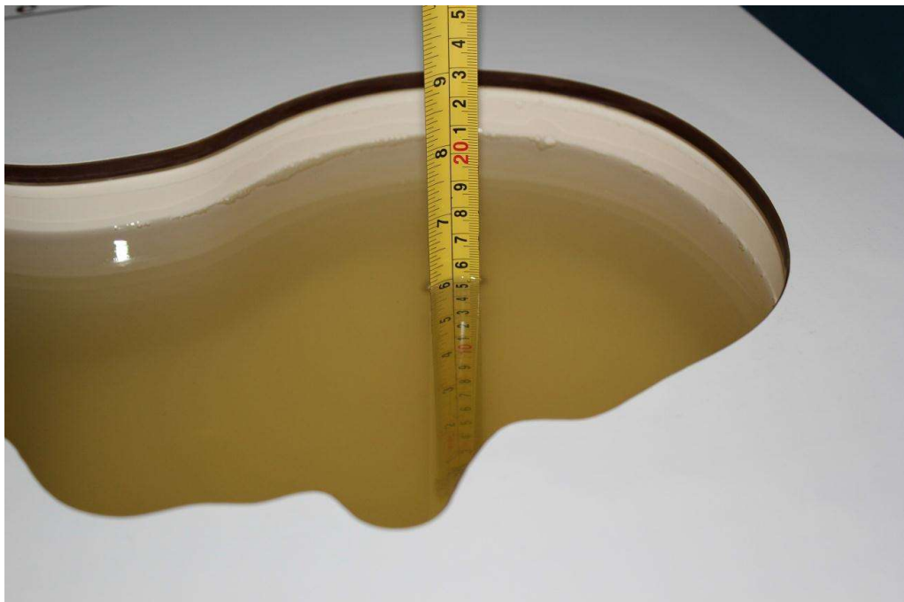
Picture 7-6: Liquid depth in the Head Phantom(2550MHz)
