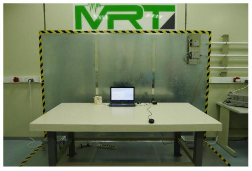
Test Mode 3 Description: Back View of Conducted Emission Test Setup
