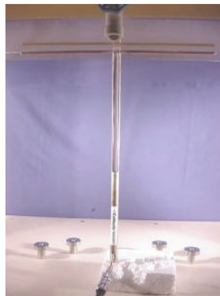
300MHz System Check Dipole Setup
