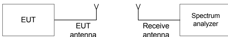
Figure 7.2.1 Carrier frequency separation test setup
