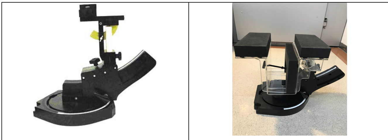
Device holder supplied by SPEAG
