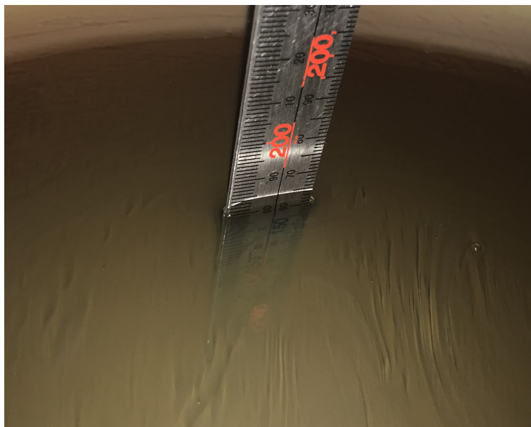
Liquid depth for SAR Measurement
