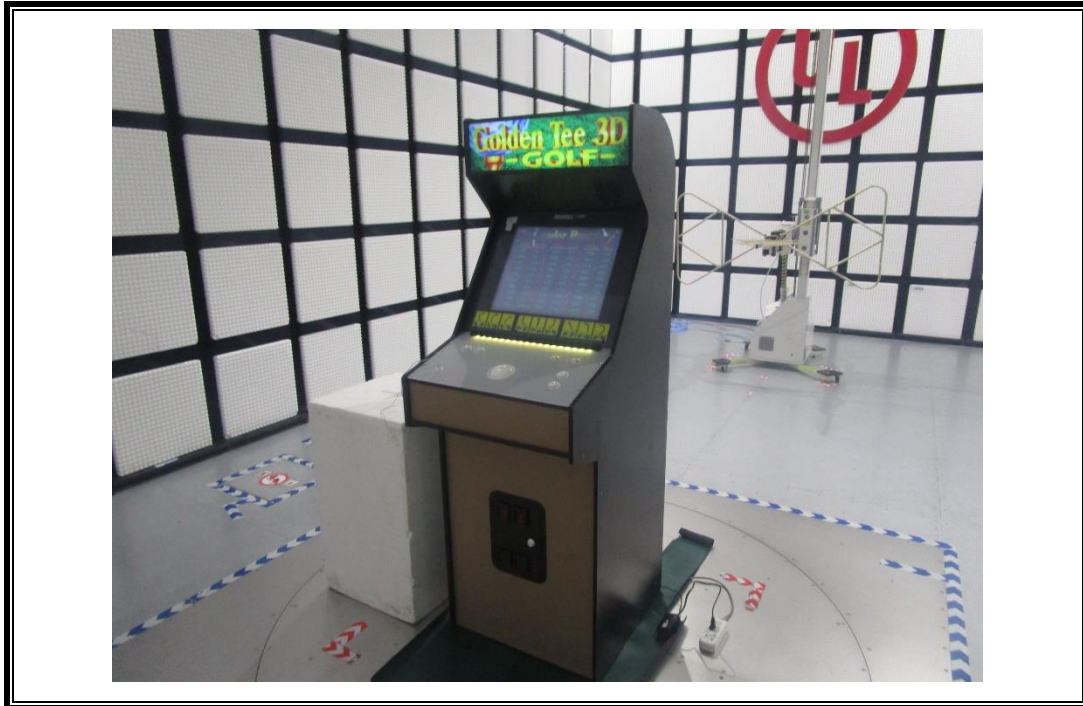
RADIATED RF MEASUREMENT SETUP (30MHz ~ 1 GHz)
