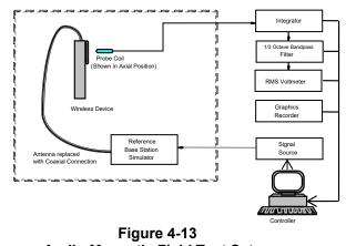
Audio Magnetic Field Test Setup
