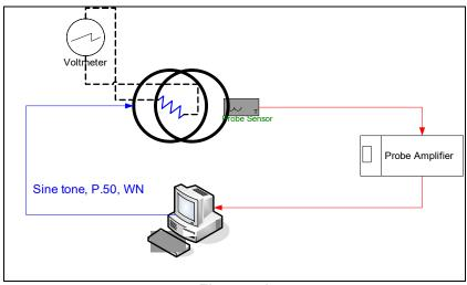
Figure 4-1 Validation Setup with Helmholtz Coil
