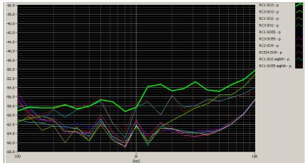
Figure 7-1 CDMA Audio Band Magnetic Noise
