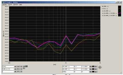
Figure 7-3 UMTS Audio Band Magnetic Noise
