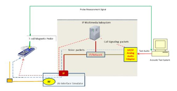
Figure 6-1 Test Setup for VoWIFI over IMS T-Coil Measurements
