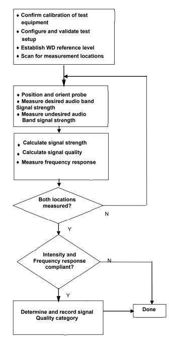
Figure 4-14 C63.19 T-Coil Signal Test Process
