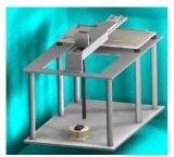
**Figure 4-3** RF Near-Field Scanner
