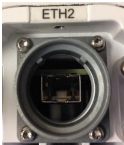
Figure 5 : Device Side Radiall OSIS Push-Pull SFP Connector
