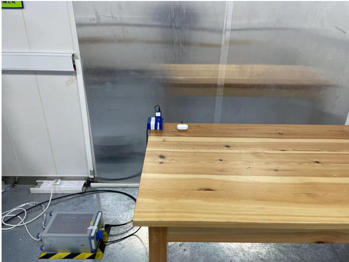
Conducted emission test setup
