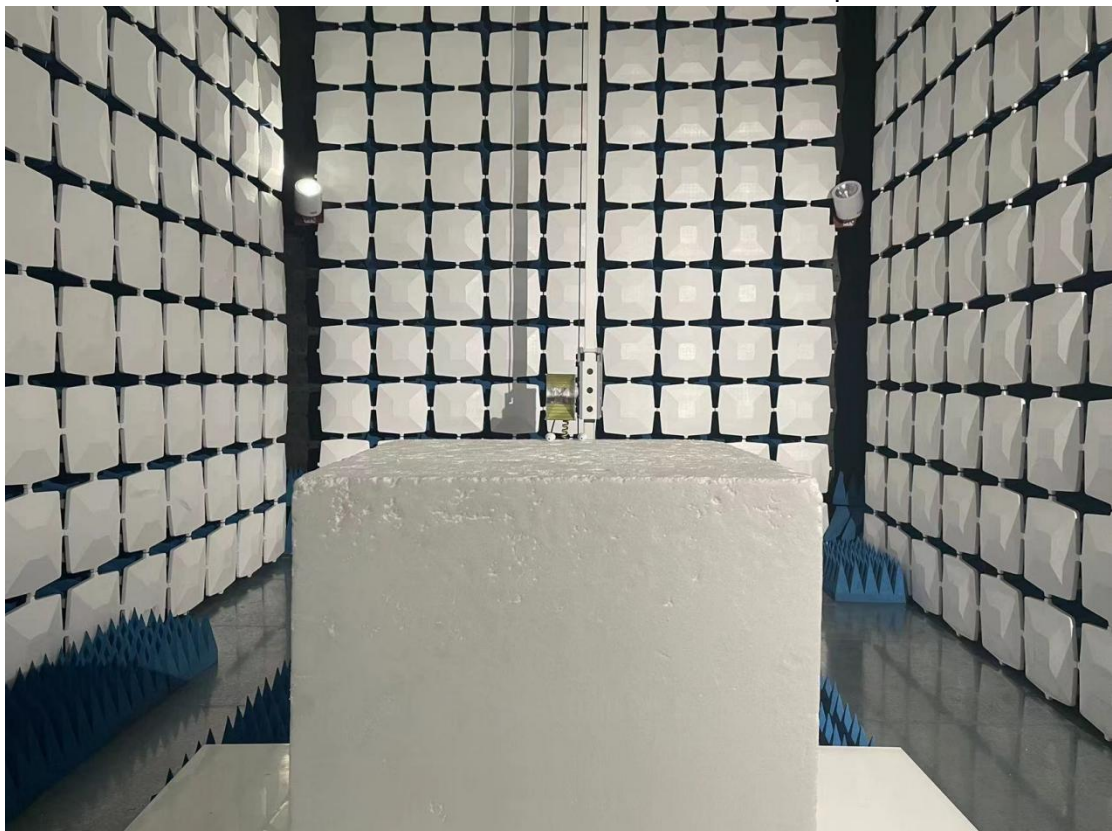
Above 1GHz for radiated emission test setup
