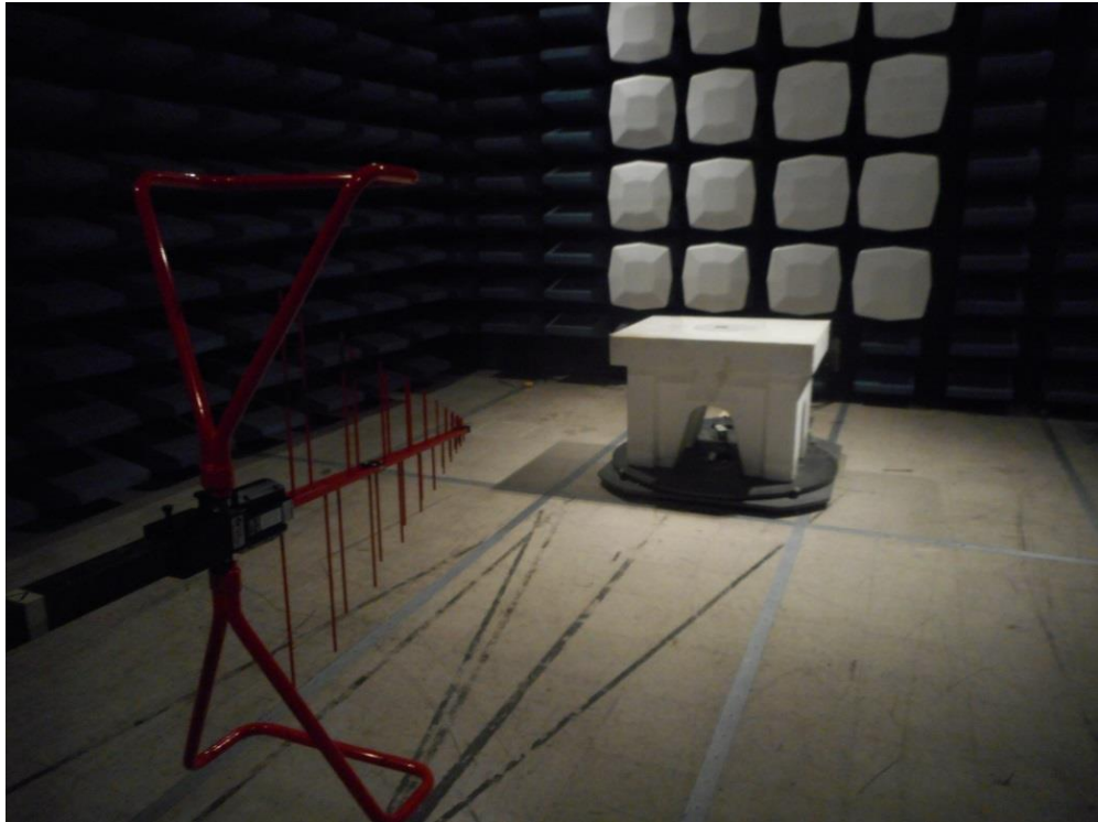
Radiated Emissions RELF 3m SAC Setup – Photo 3
