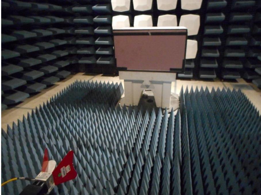
Radiated Spurious Emissions (above 1 GHz) SAC Test Setup – Photo 5
