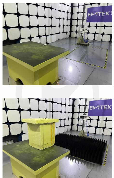
Photos Of Radiation Spurious Emission Measurement
