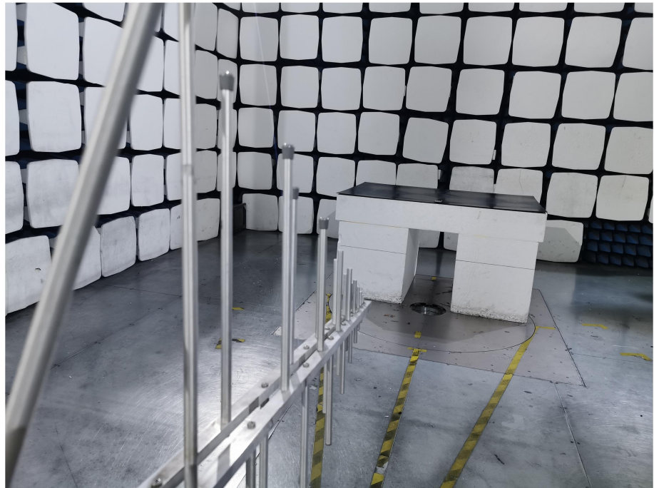
Radiation Emission Test Setup (30MHz to 1GHz)
