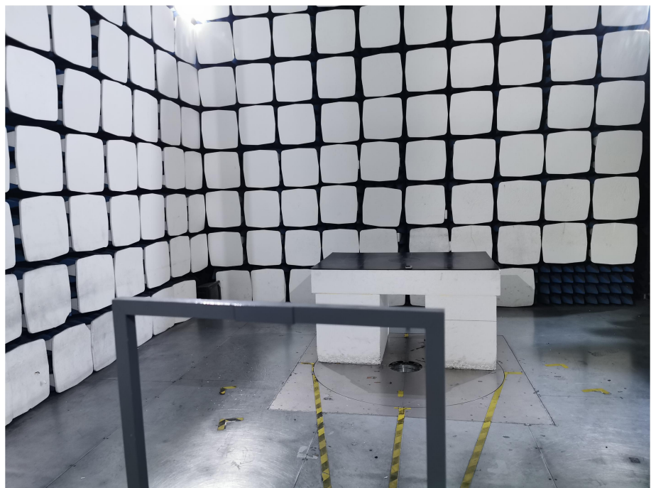
Radiation Emission Test Setup (Below 30MHz)
