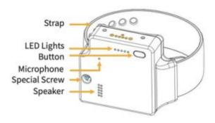
Short press the button for 1 second to power ON the tracker. The tracker can't be powered OFF by pressing button when there is SIM card installed. With SOS enabled, the wearer could short press the button for 3 seconds to trigger an SOS alert. Long press the button for 15 secondstorestart the tracker. The tracker vibrates 1 time to tell it will be restarted.
