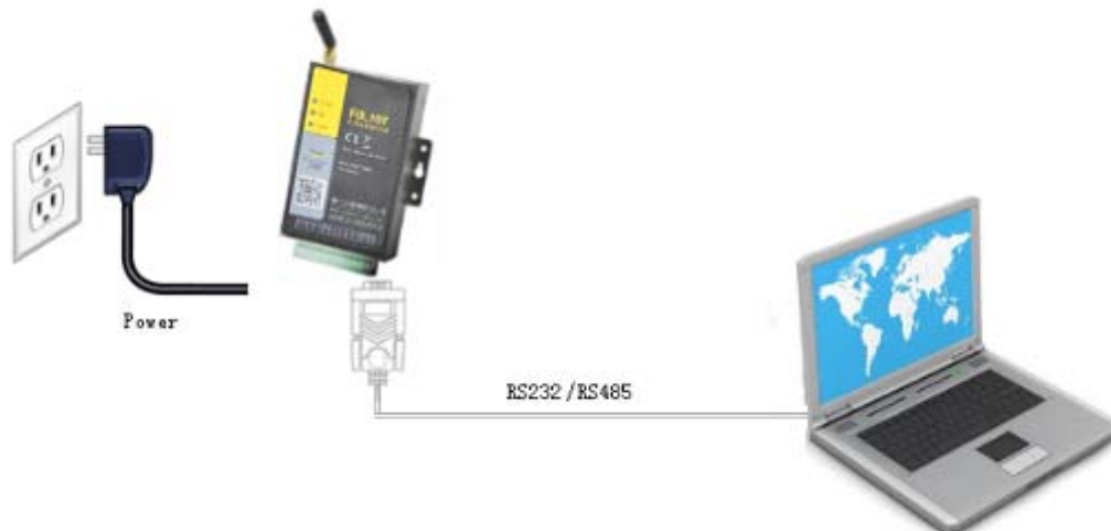
Figure 3-1 F8L10T configuration connection with PC
