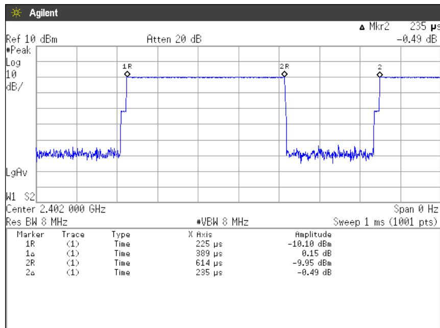
$$\text{Duty Cycle} = \text{Ton} / (\text{Ton} + \text{Toff}) = 389[\mu\text{s}] / (389[\mu\text{s}] + 235[\mu\text{s}]) = 62.34[\%]$$
