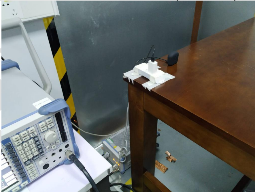
Conducted Emissions at AC Power Line (150kHz-30MHz)
