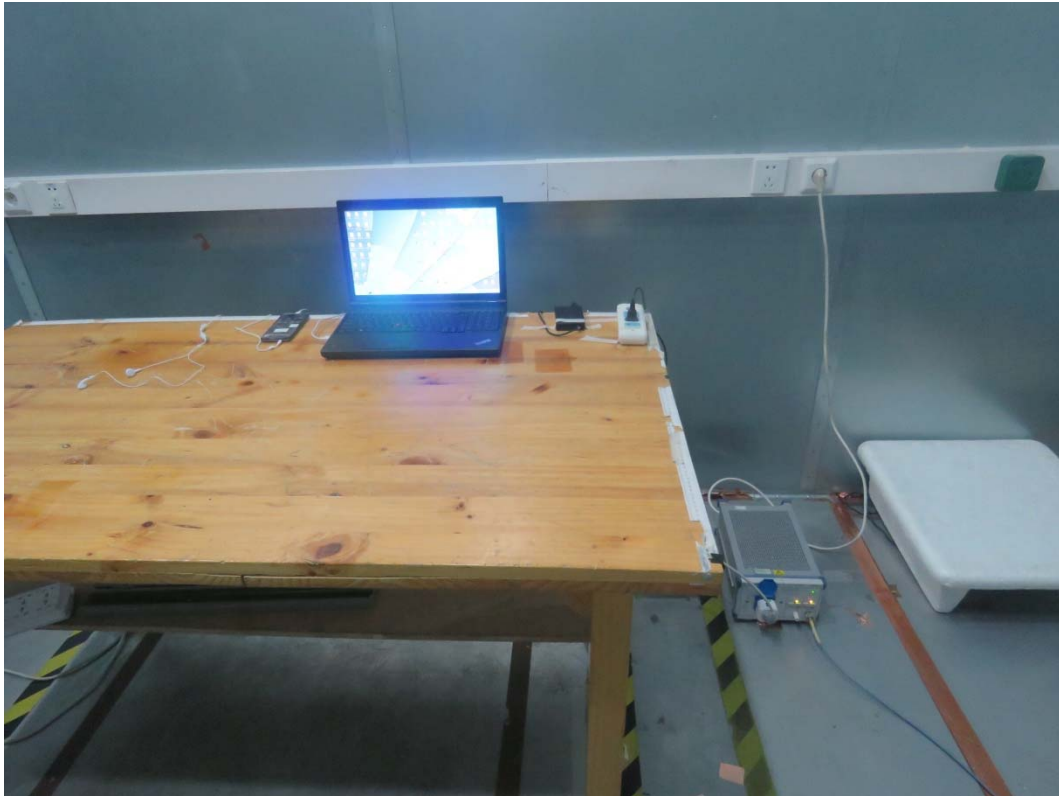
Picture 2 Conducted Emission Test Setup
