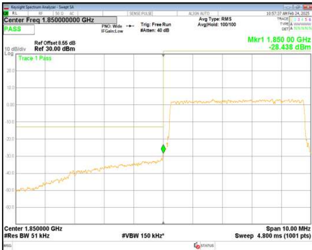
Band25 QPSK BW=5MHz Channel=26665 RB Size=25 Position=#0
