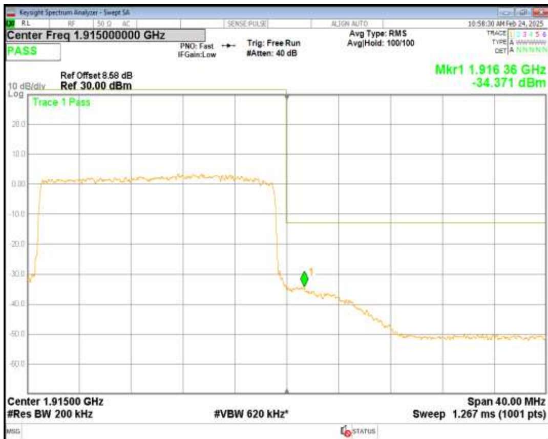
Band26(814-824) QPSK BW=1.4MHz Channel=26697 RB Size=6 Position=#0
