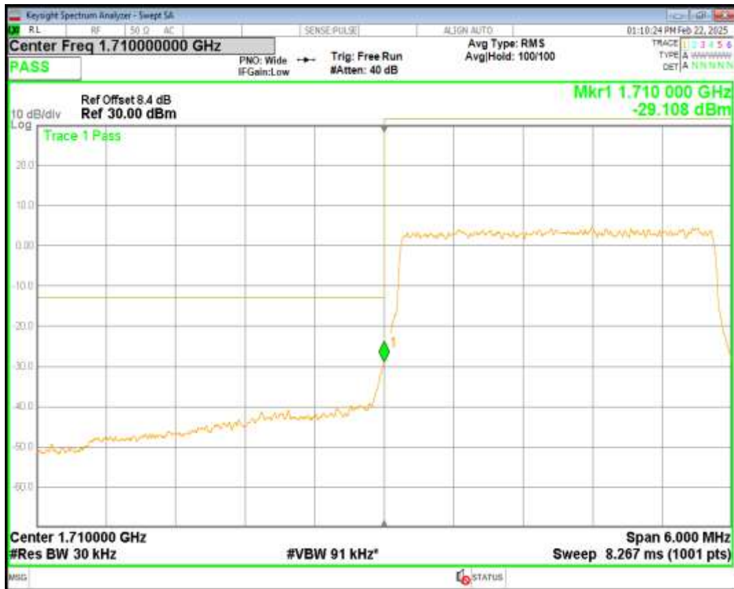
Band4 16QAM BW=3MHz Channel=19965 RB Size=15 Position=#0
