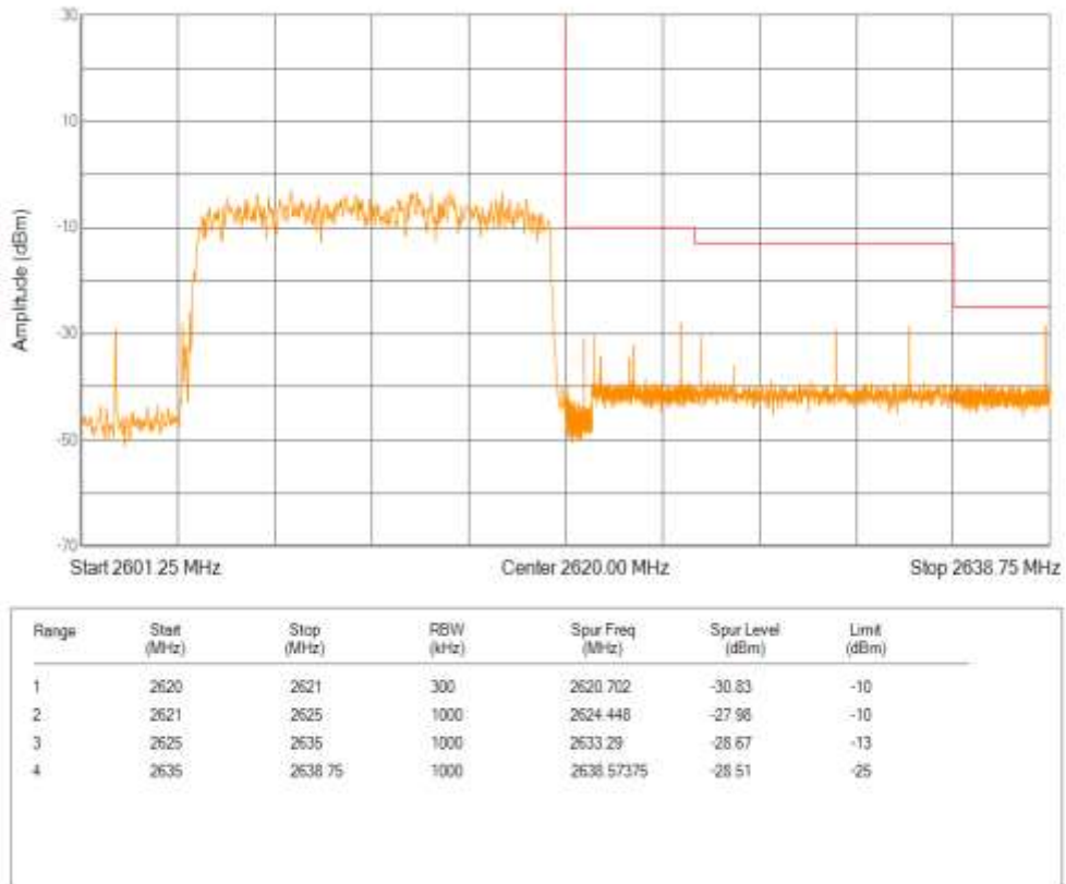
Band38 QPSK BW=5MHz Channel=37775 RB Size=25 Position=#0
