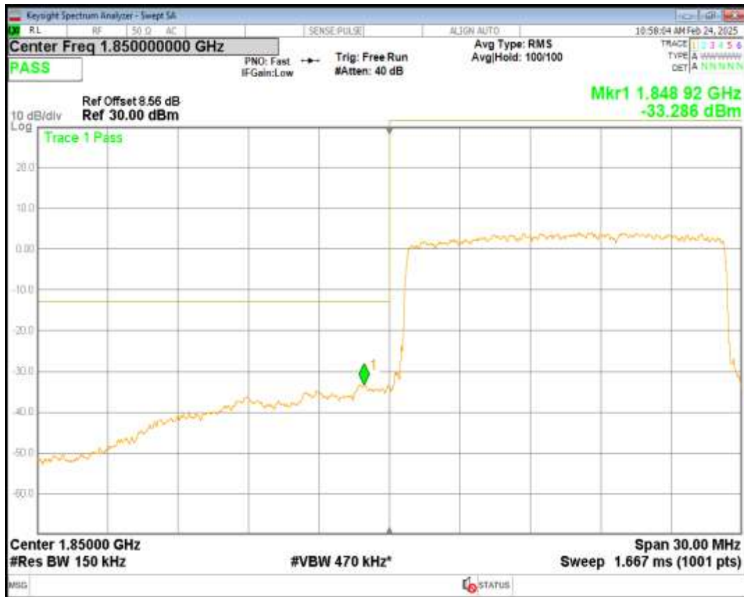
Band25 16QAM BW=15MHz Channel=26115 RB Size=75 Position=#0
