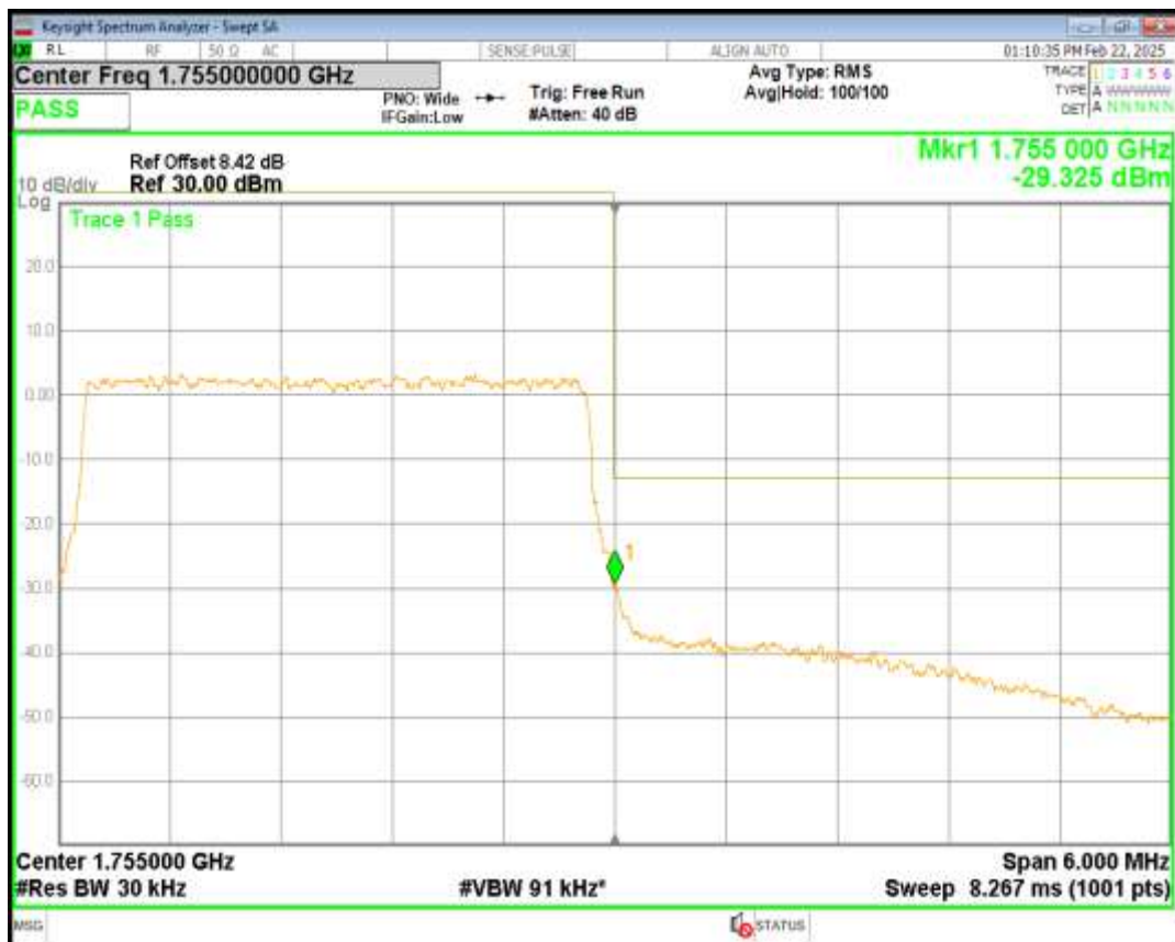
Band4 QPSK BW=5MHz Channel=19975 RB Size=25 Position=#0
