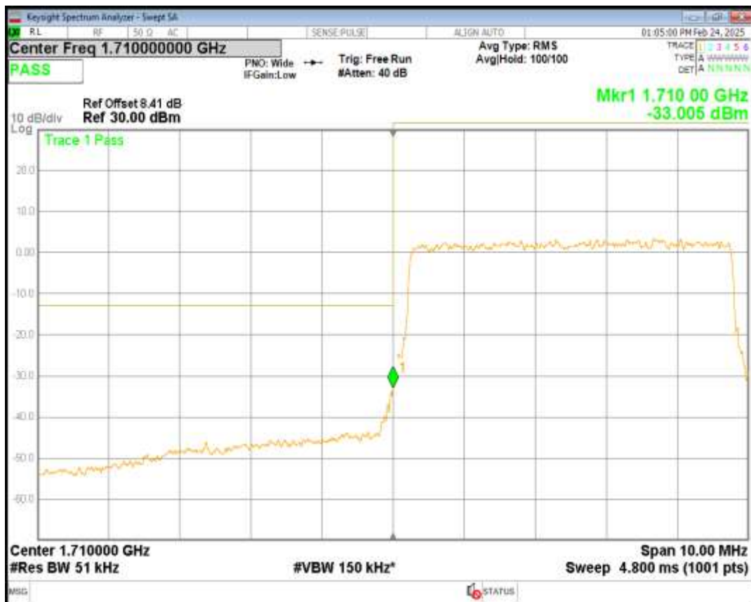
Band66 QPSK BW=5MHz Channel=132647 RB Size=25 Position=#0
