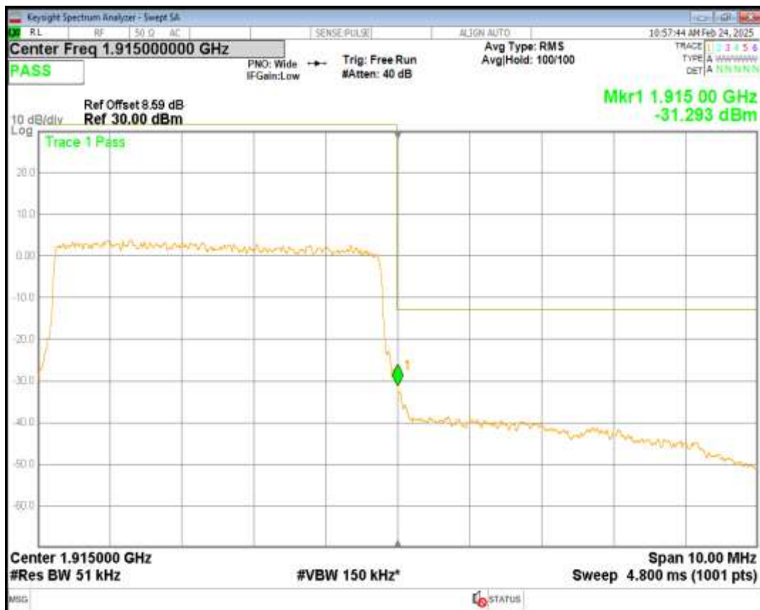
Band25 QPSK BW=10MHz Channel=26090 RB Size=50 Position=#0
