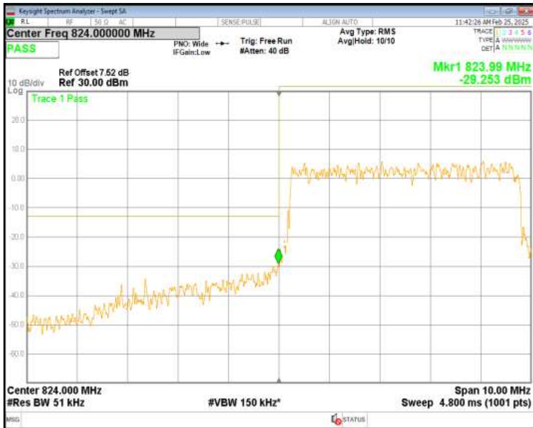
Band26(824-849) 16QAM BW=5MHz Channel=26815 RB Size=25 Position=#0
