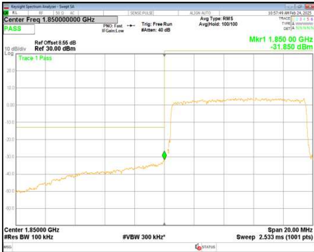
Band25 16QAM BW=10MHz Channel=26090 RB Size=50 Position=#0
