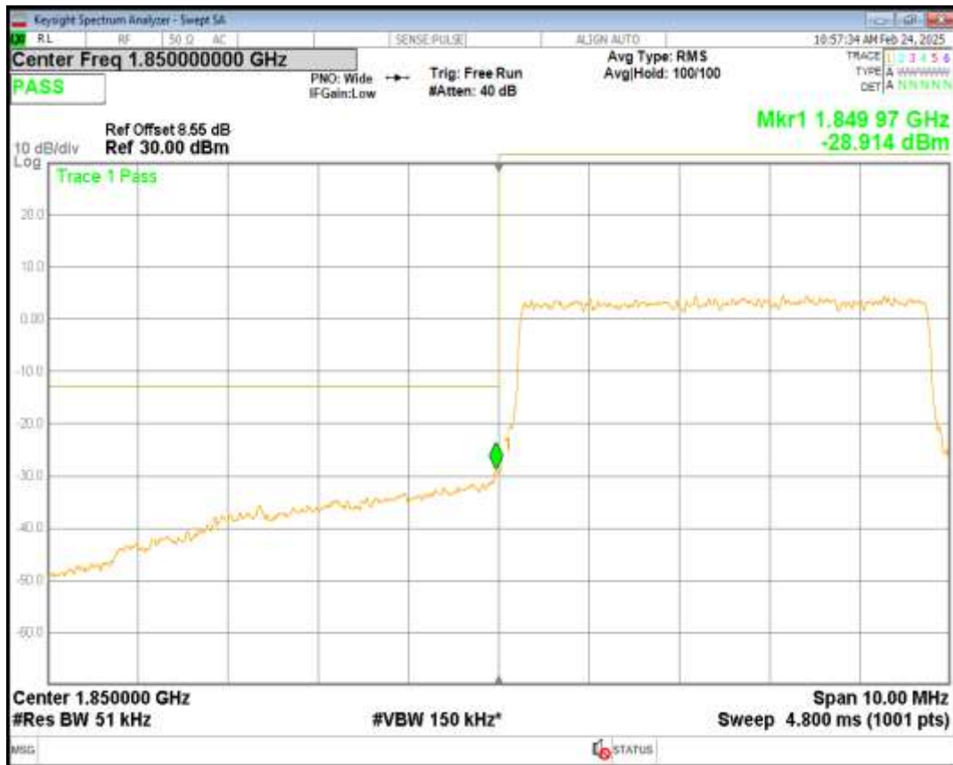
Band25 16QAM BW=5MHz Channel=26065 RB Size=25 Position=#0
