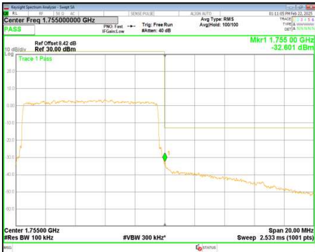
Band4 QPSK BW=15MHz Channel=20025 RB Size=75 Position=#0
