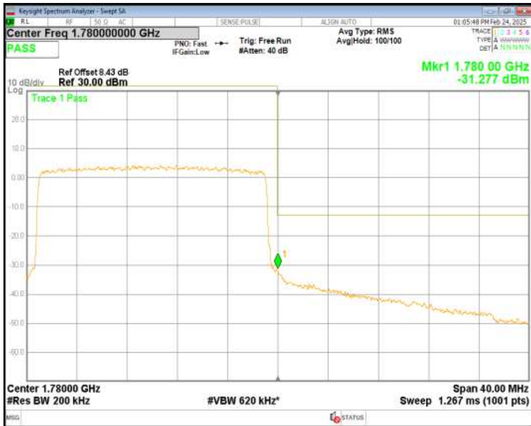
Band66 16QAM BW=20MHz Channel=132572 RB Size=100 Position=#0
