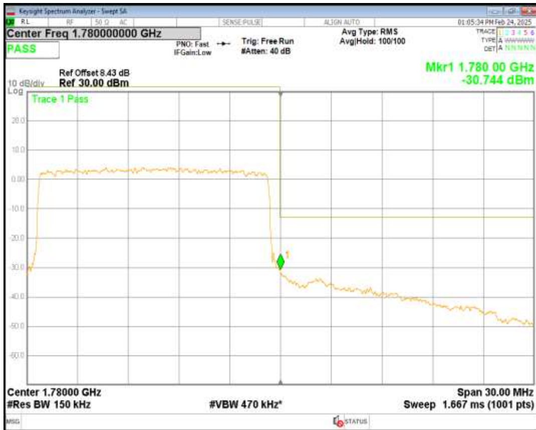
Band66 16QAM BW=15MHz Channel=132597 RB Size=75 Position=#0
