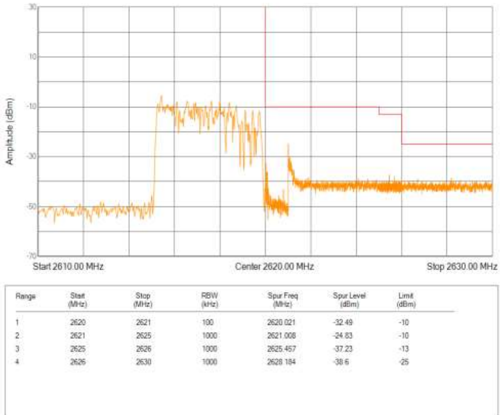
Band38 QPSK BW=10MHz Channel=37800 RB Size=50 Position=#0
