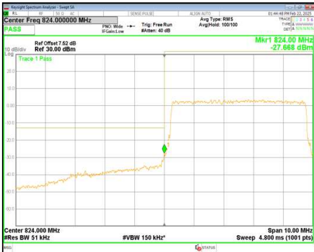
Band5 QPSK BW=5MHz Channel=20625 RB Size=25 Position=#0
