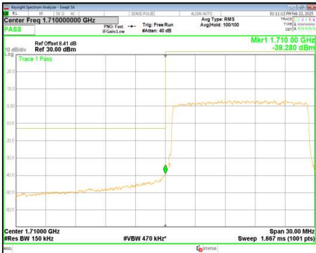
Band4 QPSK BW=15MHz Channel=20325 RB Size=75 Position=#0
