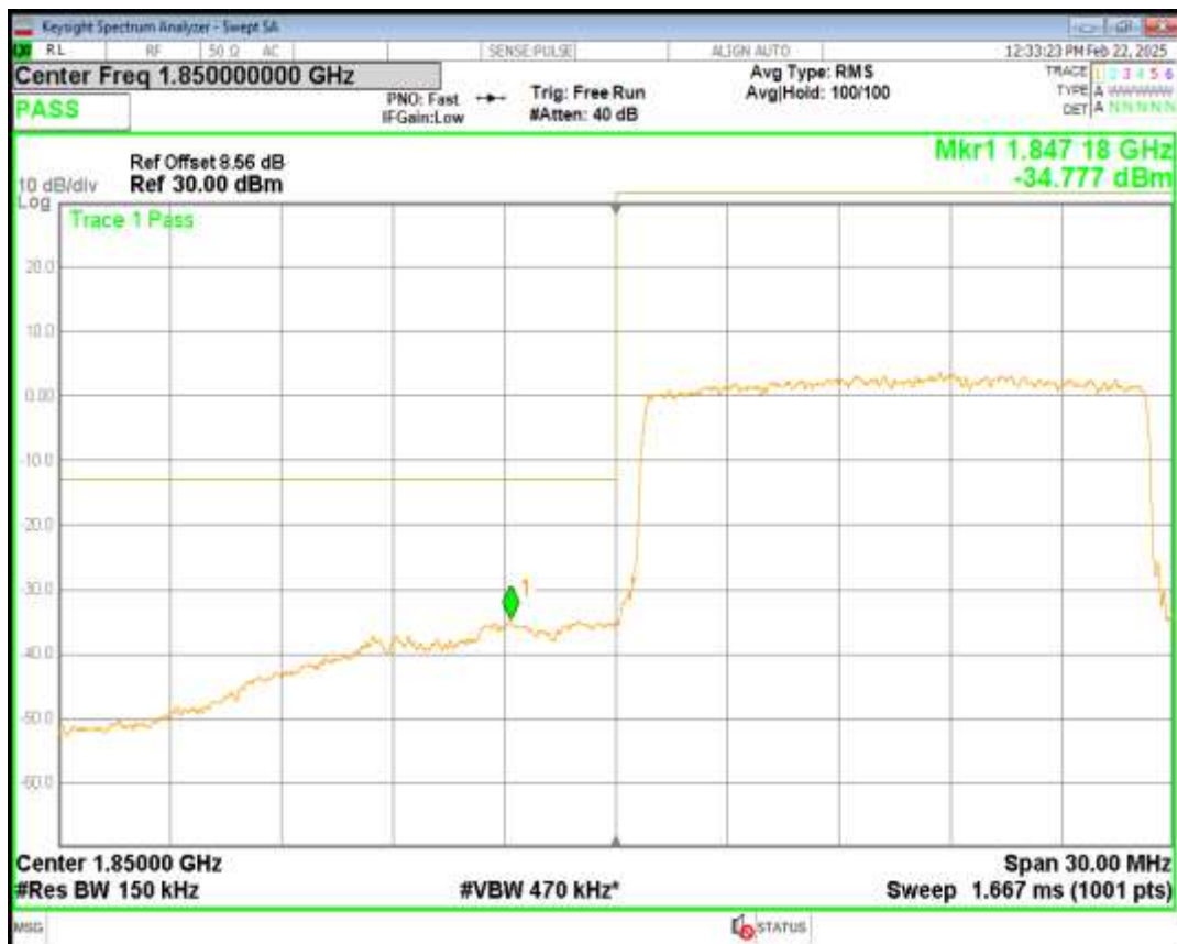
Band2 QPSK BW=15MHz Channel=19125 RB Size=75 Position=#0
