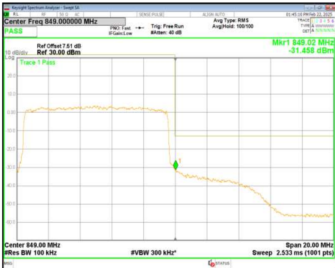
Band66 QPSK BW=1.4MHz Channel=131979 RB Size=6 Position=#0
