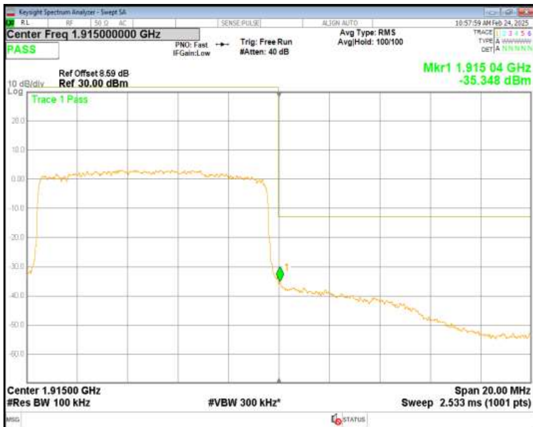
Band25 QPSK BW=15MHz Channel=26115 RB Size=75 Position=#0
