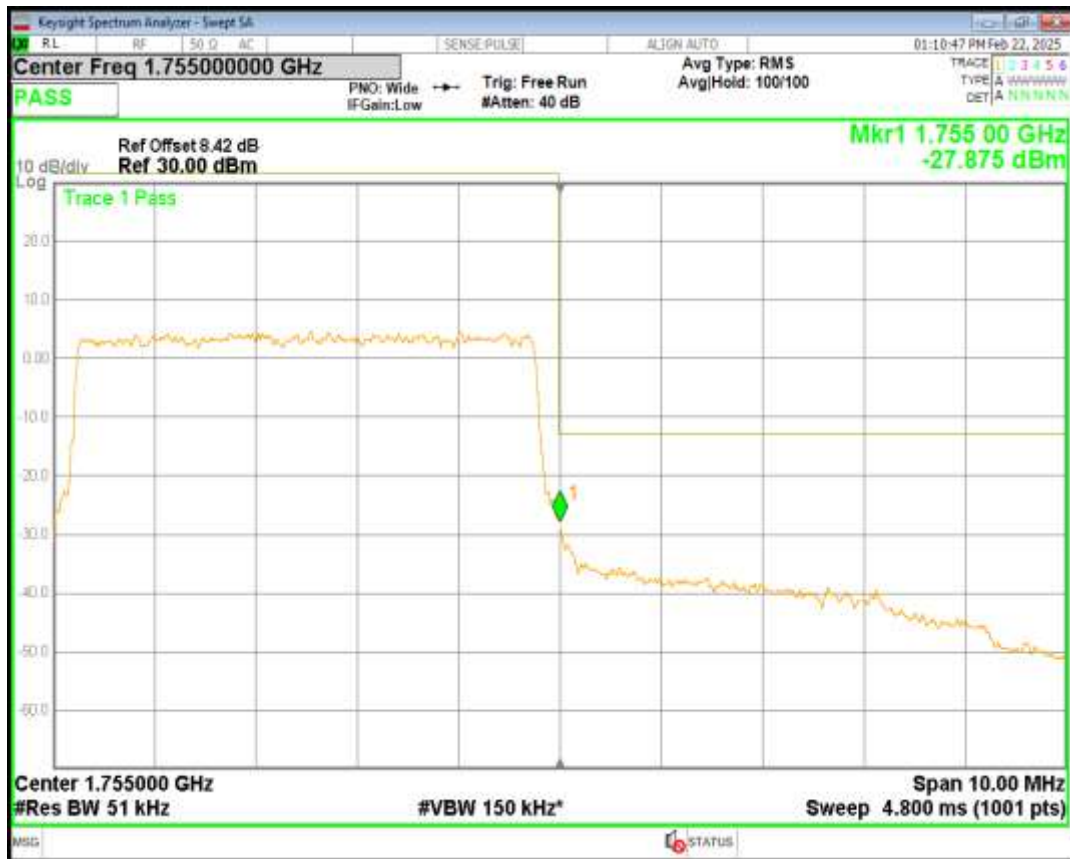
Band4 16QAM BW=5MHz Channel=20375 RB Size=25 Position=#0
