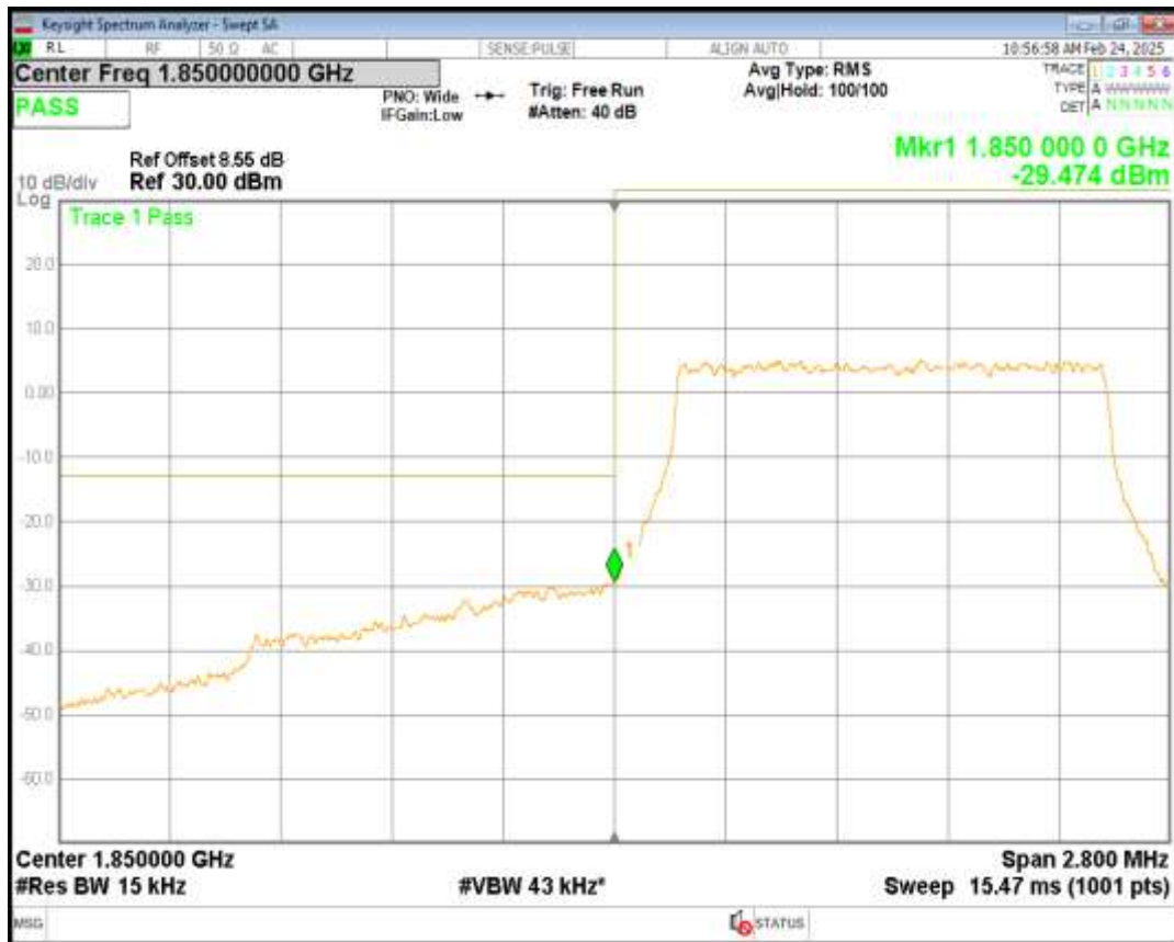
Band25 16QAM BW=1.4MHz Channel=26047 RB Size=6 Position=#0
