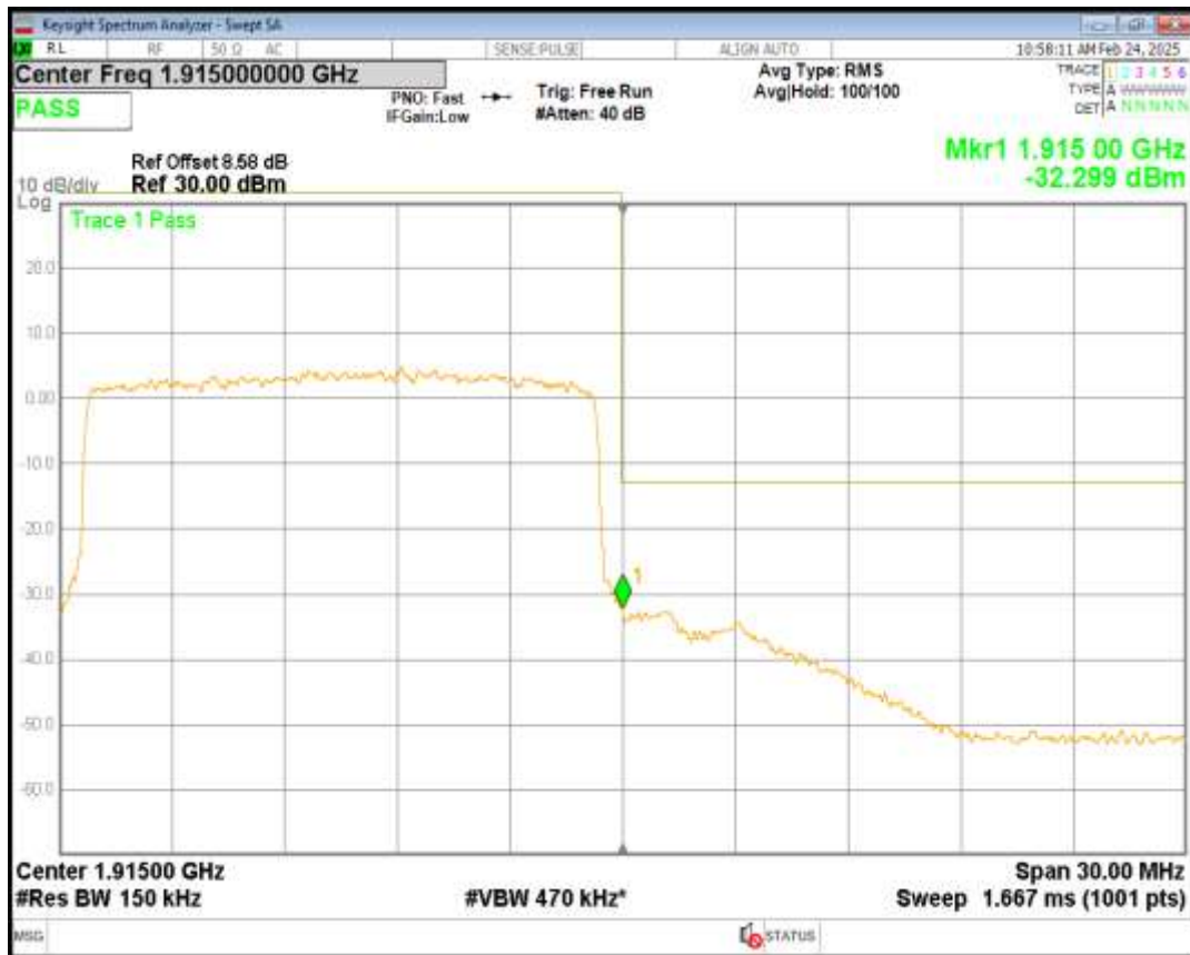
Band25 16QAM BW=15MHz Channel=26615 RB Size=75 Position=#0
