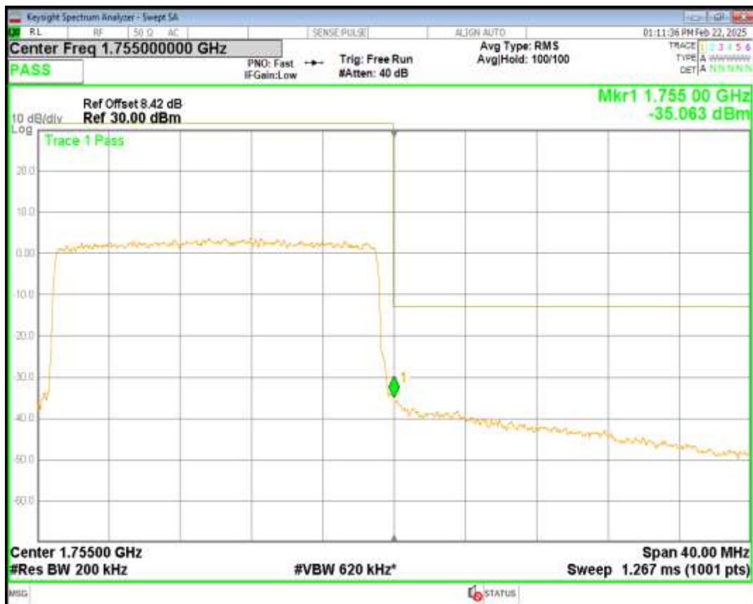
Band41 QPSK BW=5MHz Channel=39675 RB Size=25 Position=#0
