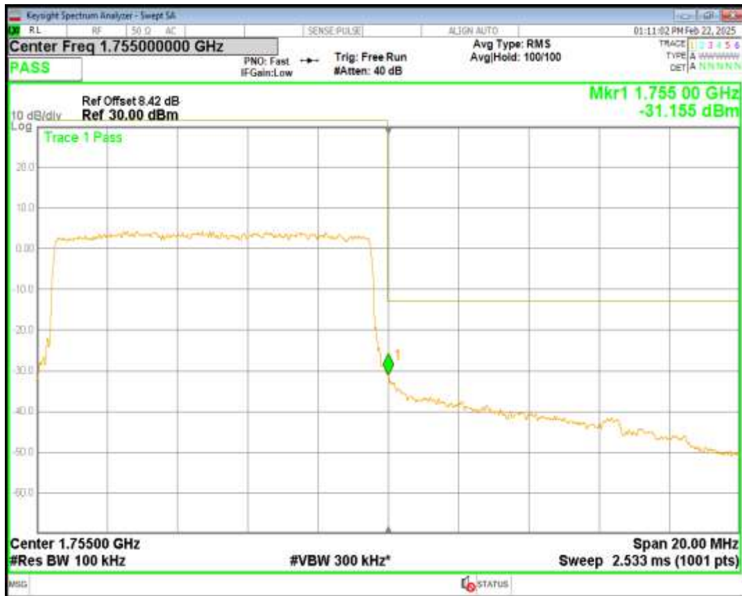
Band4 16QAM BW=10MHz Channel=20350 RB Size=50 Position=#0
