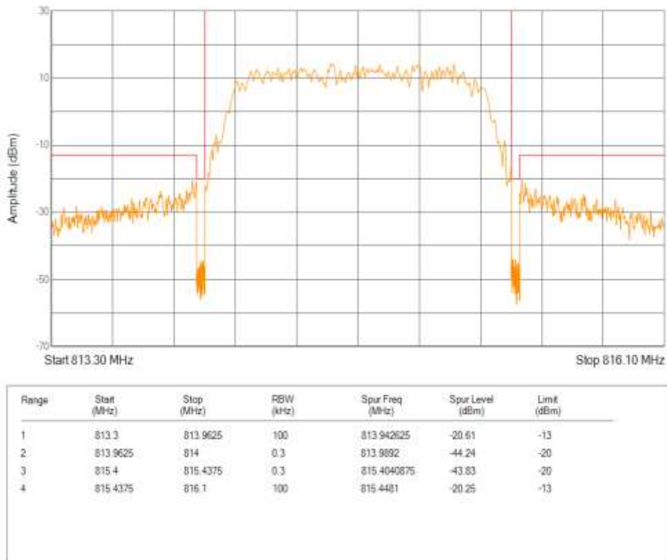
Band26(814-824) QPSK BW=1.4MHz Channel=26783 RB Size=6 Position=#0
