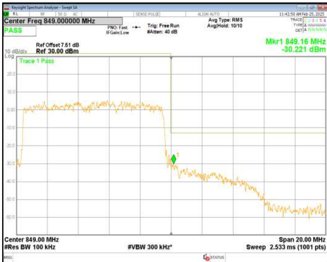
Band26(824-849) QPSK BW=15MHz Channel=26865 RB Size=75 Position=#0
