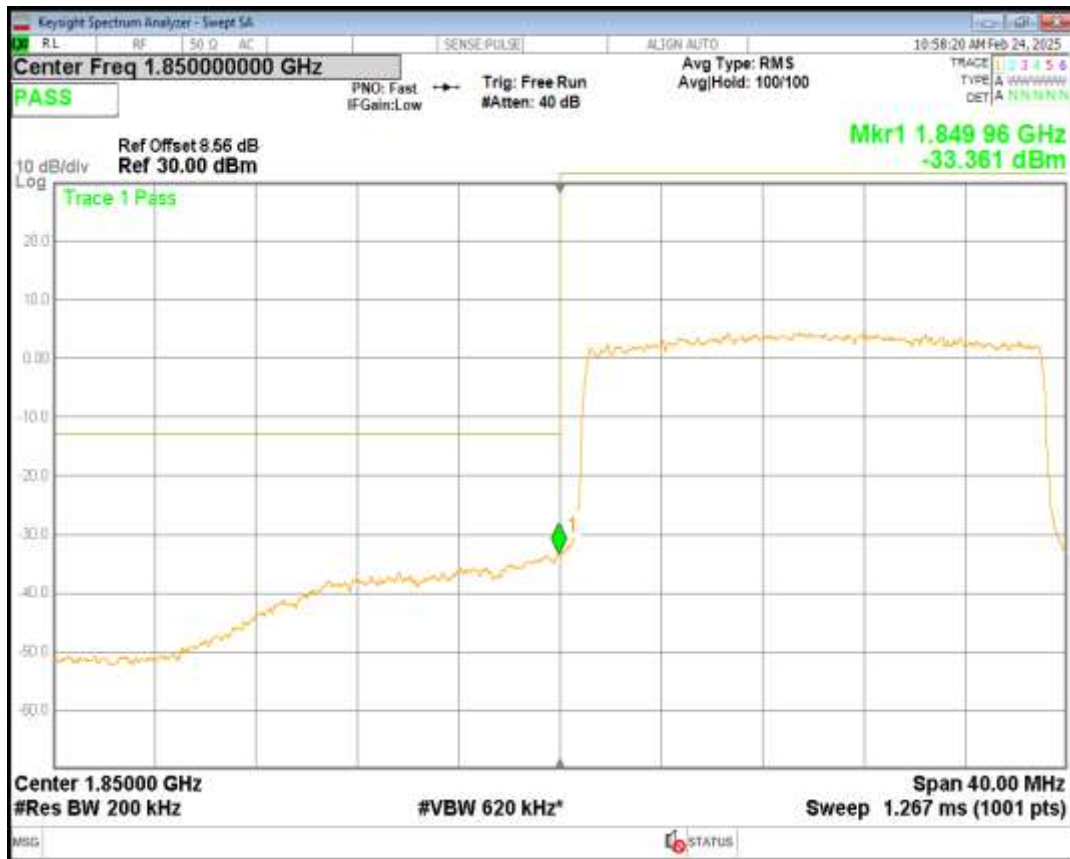
Band25 16QAM BW=20MHz Channel=26140 RB Size=100 Position=#0
