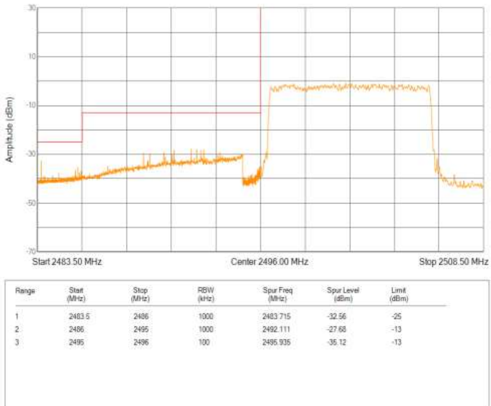
Band41 QPSK BW=10MHz Channel=41540 RB Size=50 Position=#0
