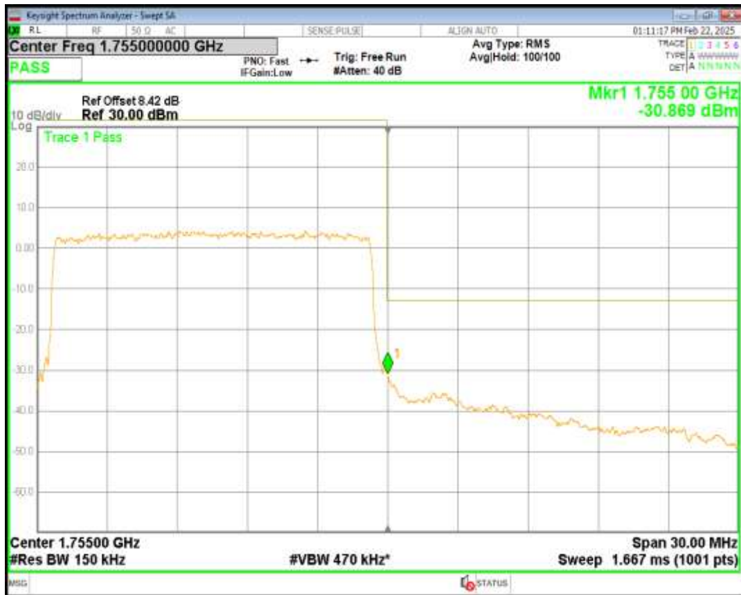
Band4 16QAM BW=15MHz Channel=20325 RB Size=75 Position=#0
