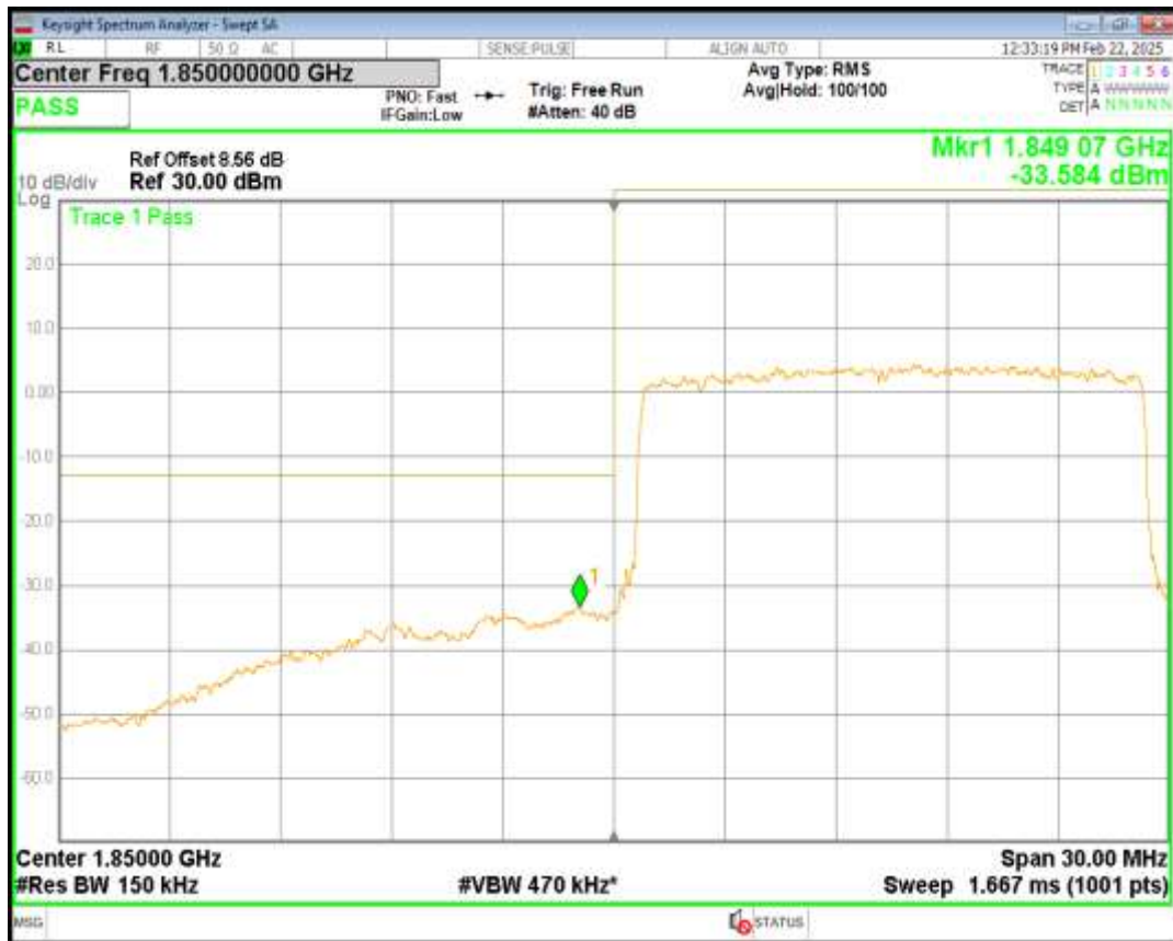
Band2 16QAM BW=15MHz Channel=18675 RB Size=75 Position=#0
