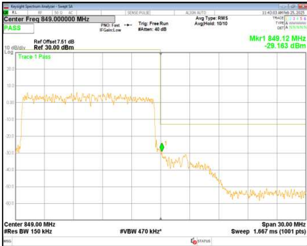
Band26(824-849) 16QAM BW=15MHz Channel=26965 RB Size=75 Position=#0
