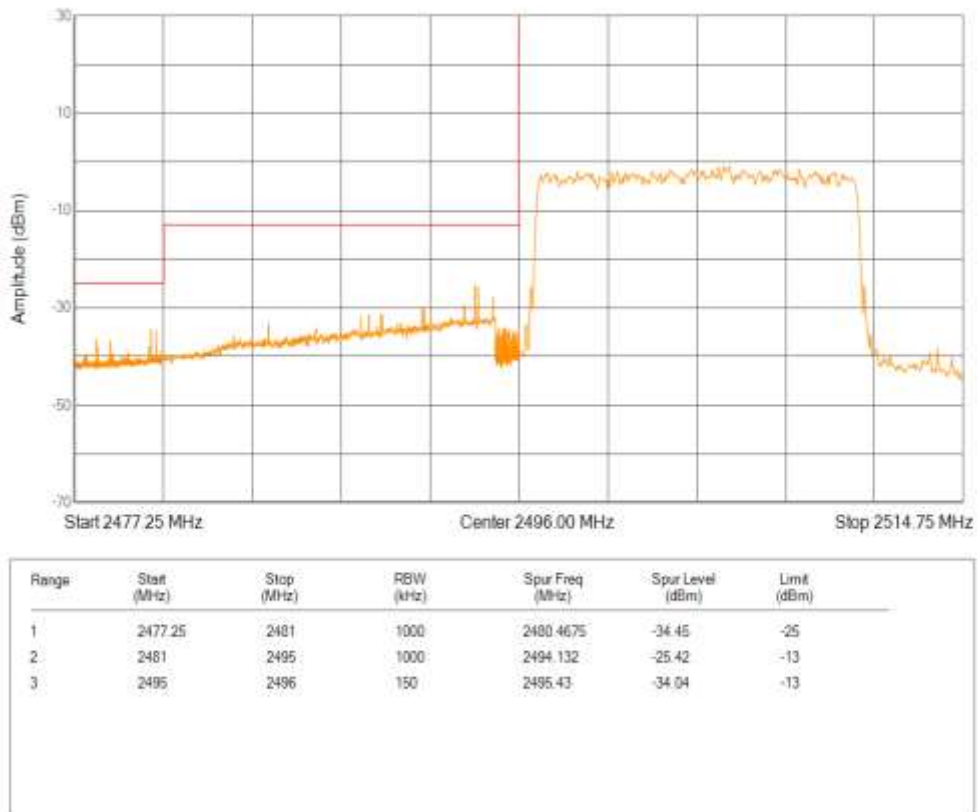
Band41 QPSK BW=15MHz Channel=41515 RB Size=75 Position=#0
