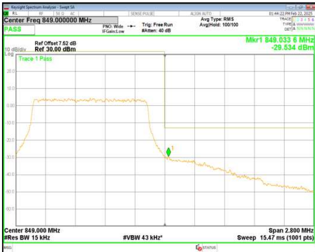
Band5 QPSK BW=3MHz Channel=20415 RB Size=15 Position=#0
