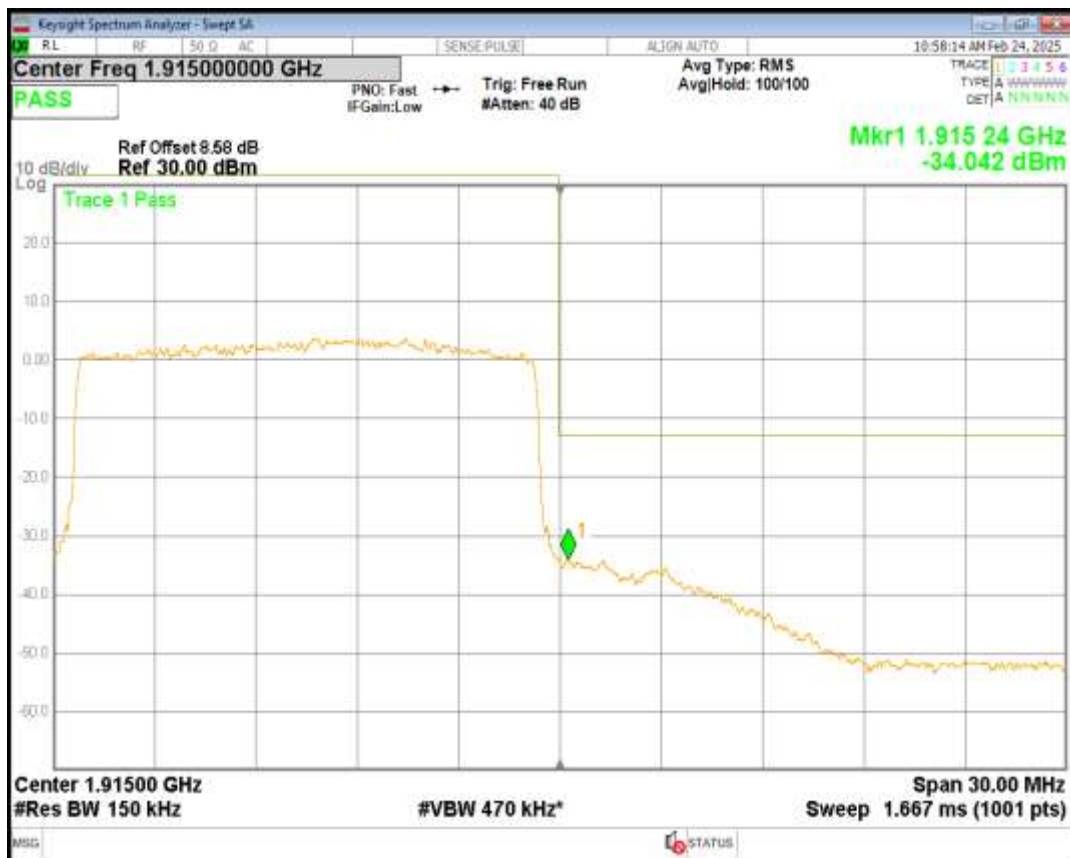
Band25 QPSK BW=20MHz Channel=26140 RB Size=100 Position=#0
