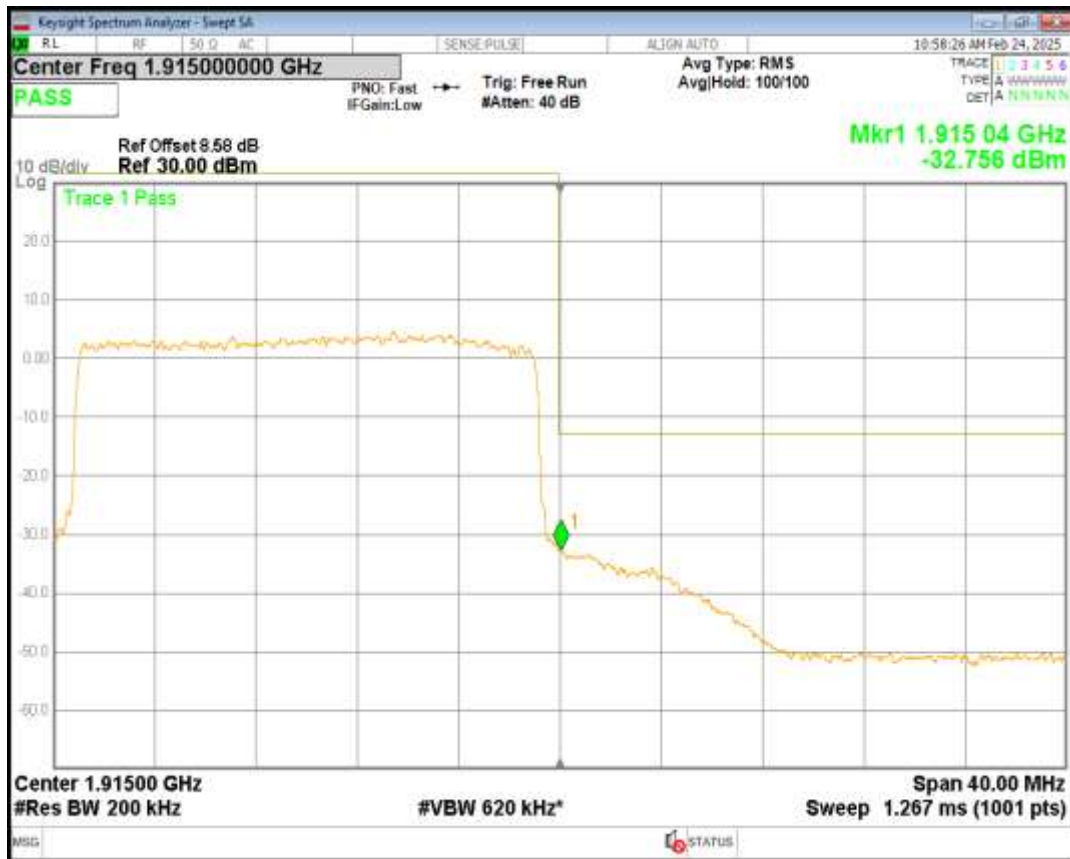
Band25 16QAM BW=20MHz Channel=26590 RB Size=100 Position=#0
