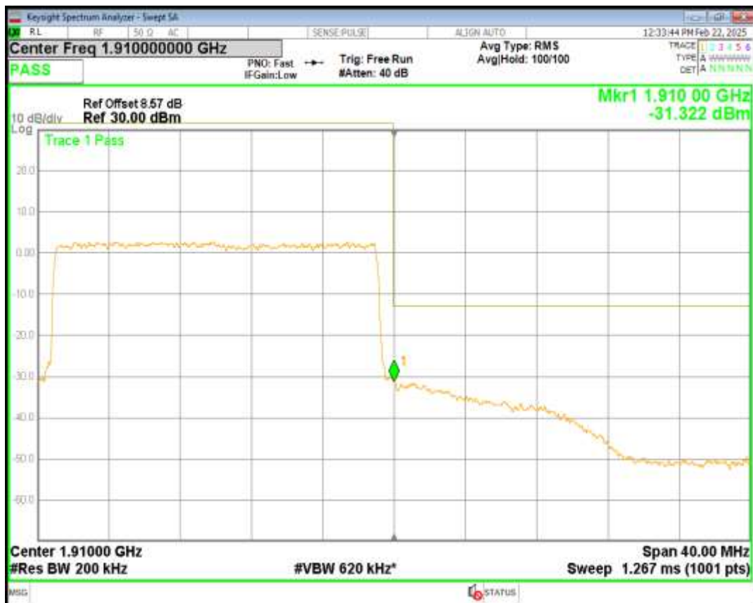
Band25 QPSK BW=1.4MHz Channel=26047 RB Size=6 Position=#0
