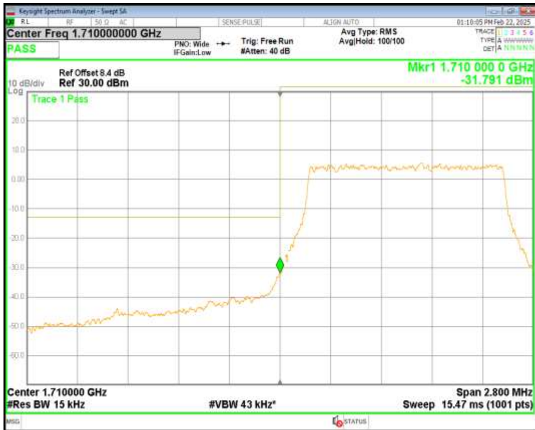
Band4 16QAM BW=1.4MHz Channel=19957 RB Size=6 Position=#0
