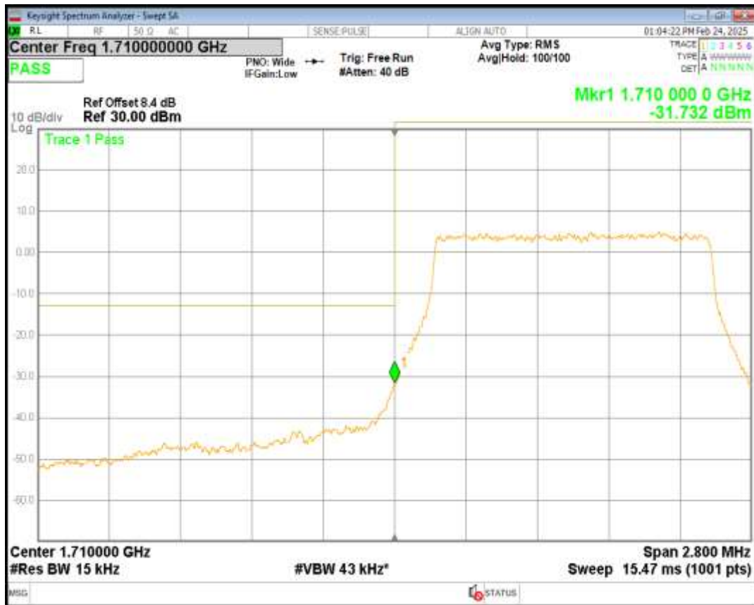
Band66 16QAM BW=1.4MHz Channel=131979 RB Size=6 Position=#0
