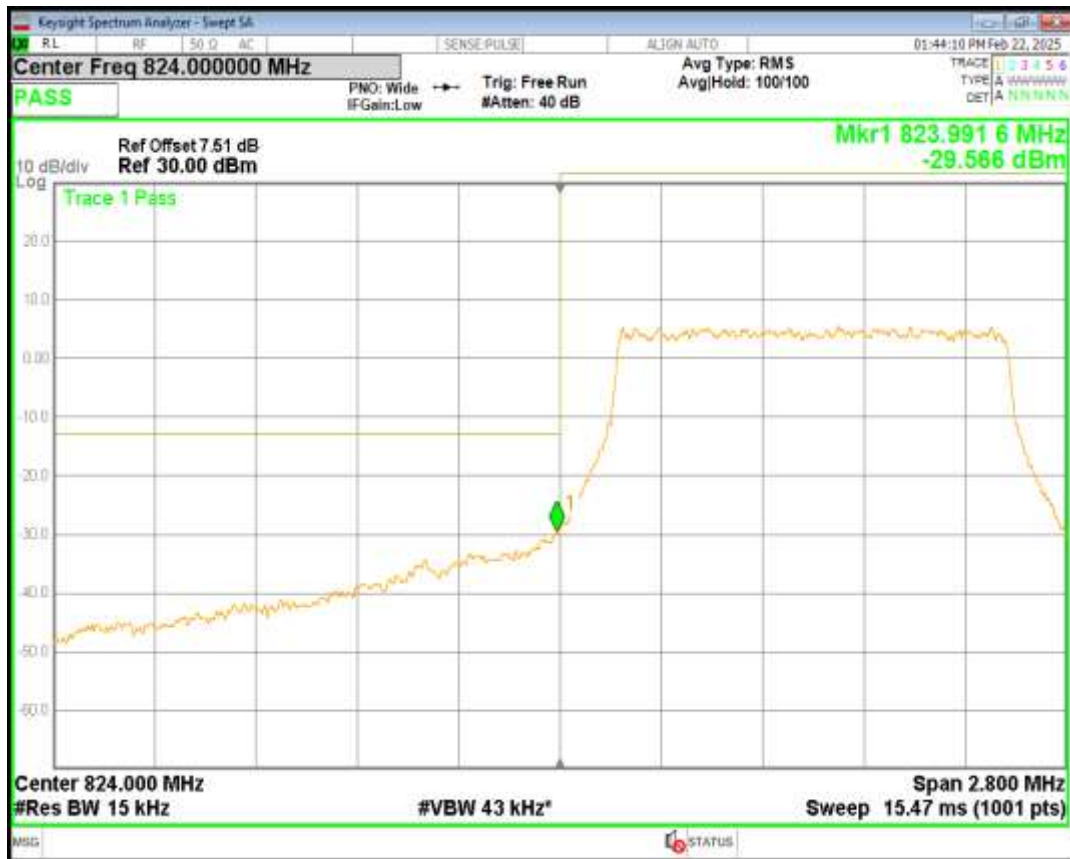
Band5 16QAM BW=1.4MHz Channel=20407 RB Size=6 Position=#0
