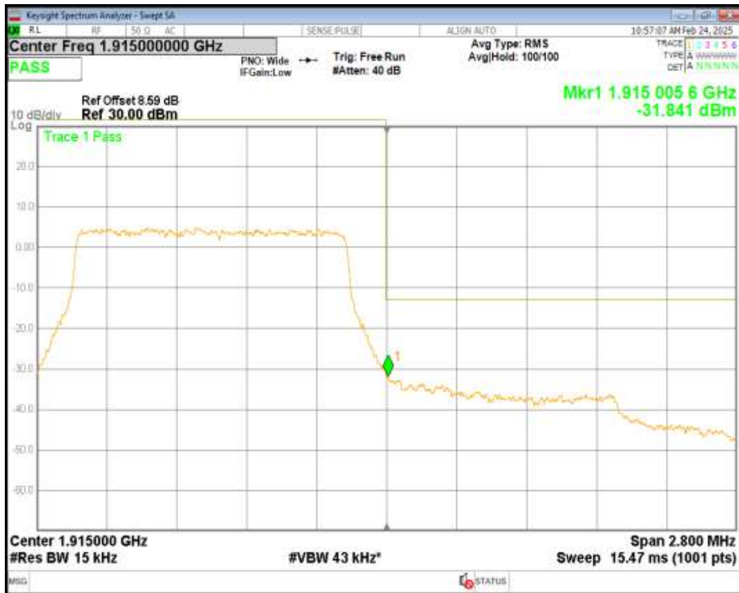
Band25 16QAM BW=1.4MHz Channel=26683 RB Size=6 Position=#0
