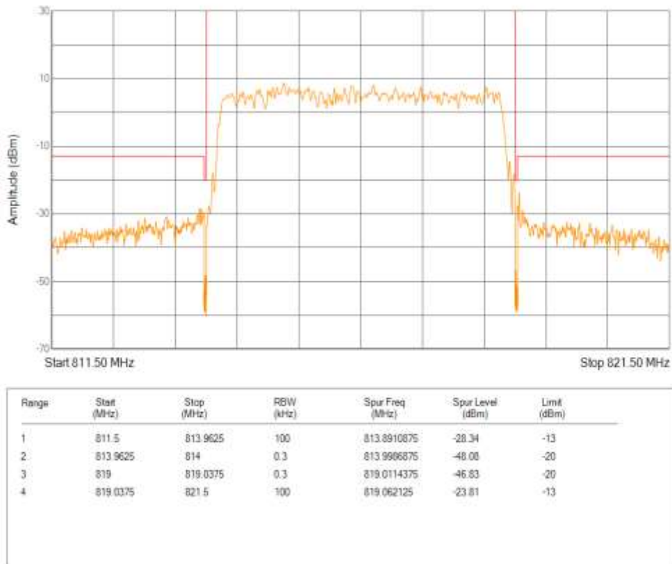
Band26(814-824) QPSK BW=5MHz Channel=26765 RB Size=25 Position=#0
