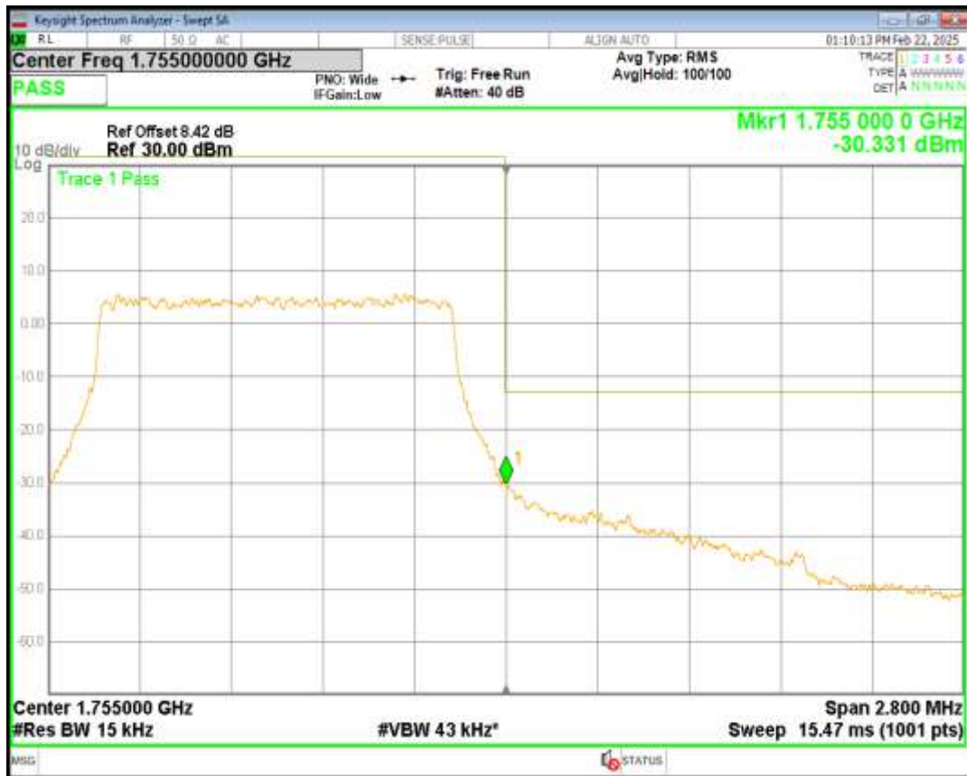
Band4 16QAM BW=1.4MHz Channel=20393 RB Size=6 Position=#0
