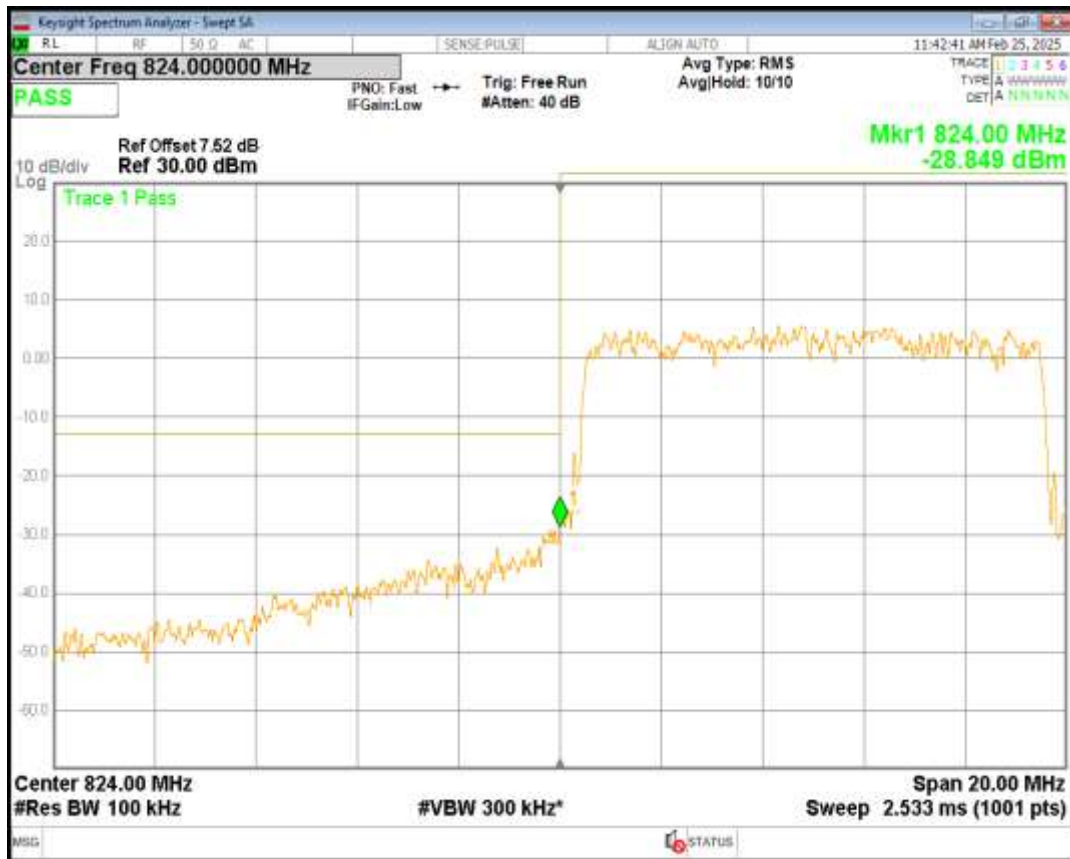
Band26(824-849) 16QAM BW=10MHz Channel=26840 RB Size=50 Position=#0
