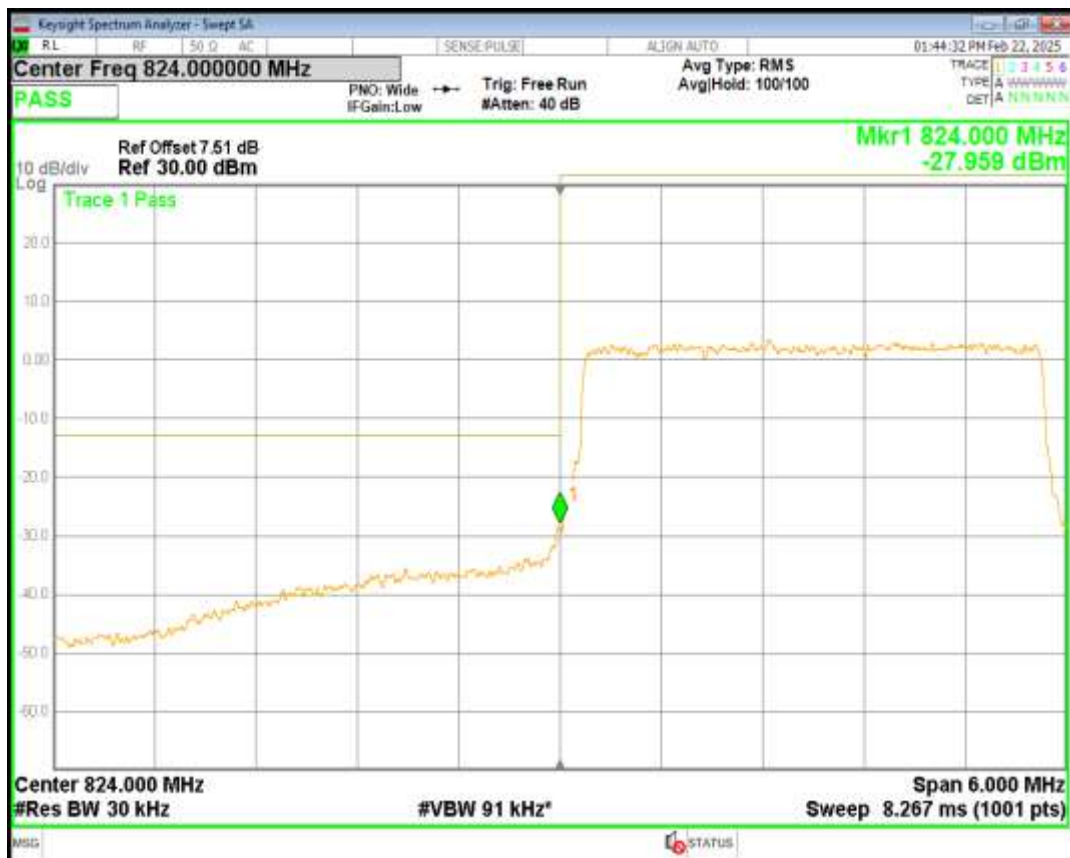
Band5 QPSK BW=3MHz Channel=20635 RB Size=15 Position=#0
