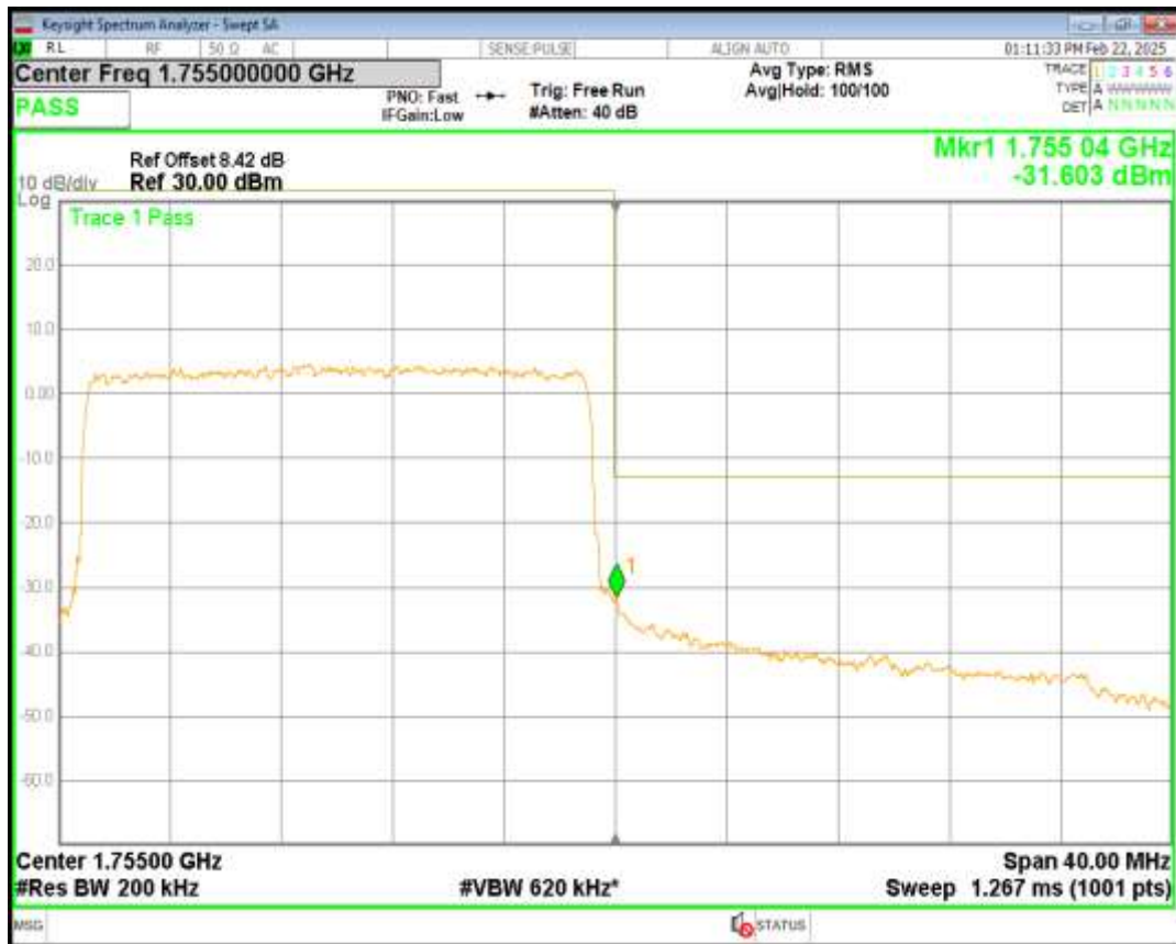
Band4 16QAM BW=20MHz Channel=20300 RB Size=100 Position=#0
