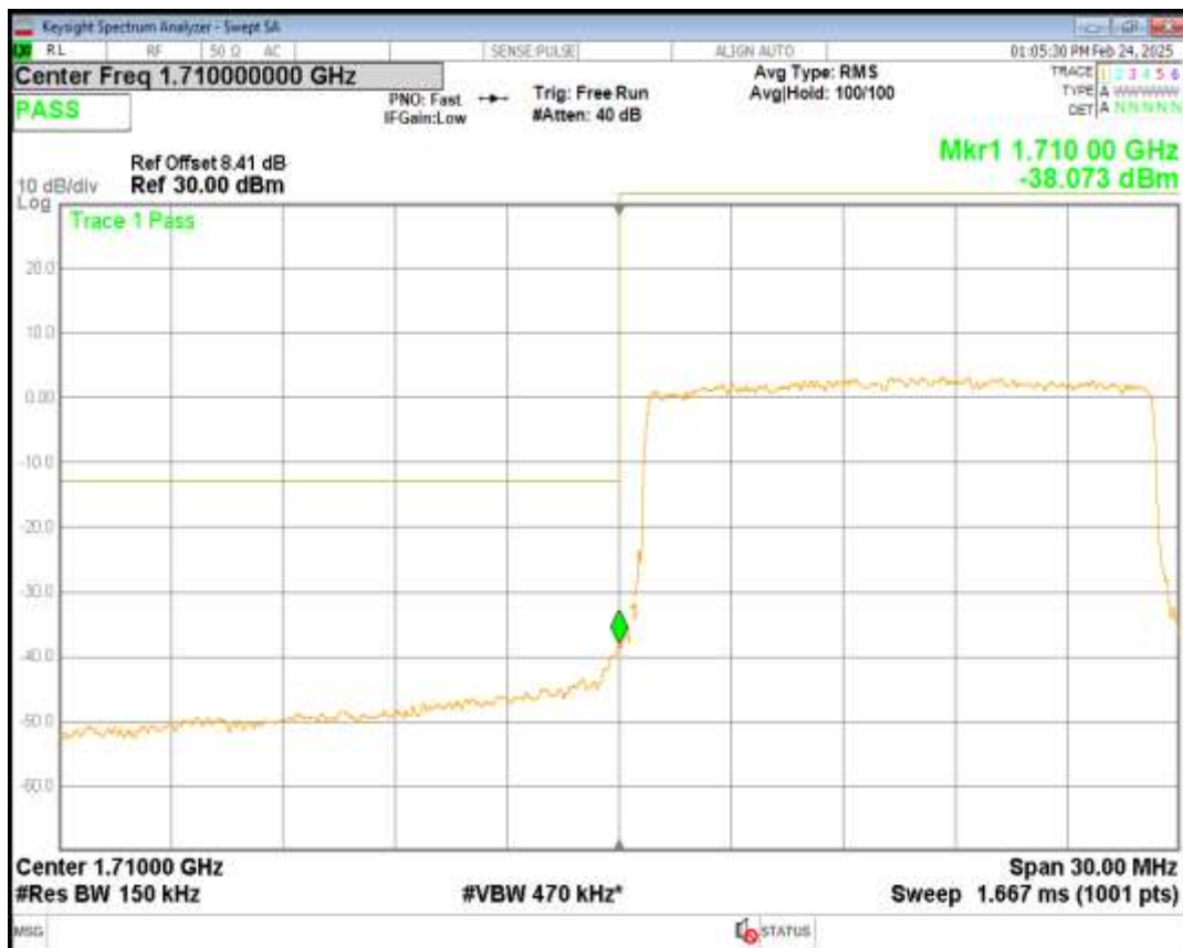
Band66 QPSK BW=15MHz Channel=132597 RB Size=75 Position=#0
