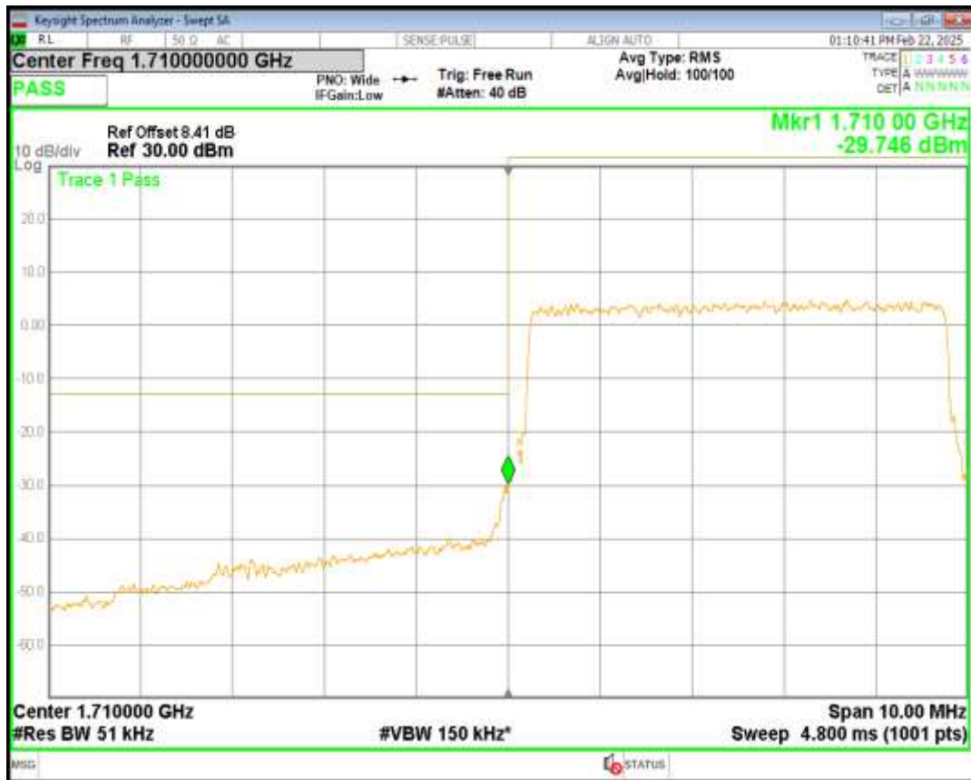
Band4 16QAM BW=5MHz Channel=19975 RB Size=25 Position=#0
