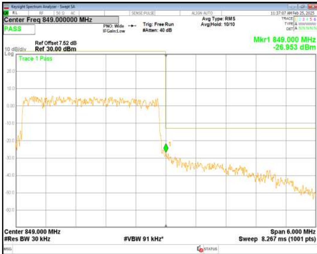
Band26(824-849) 16QAM BW=3MHz Channel=27025 RB Size=15 Position=#0
