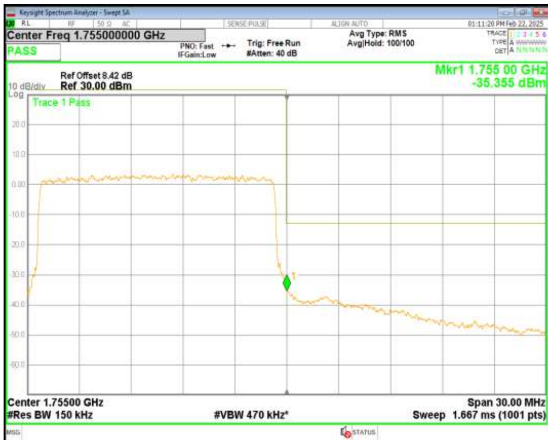
Band4 QPSK BW=20MHz Channel=20050 RB Size=100 Position=#0
