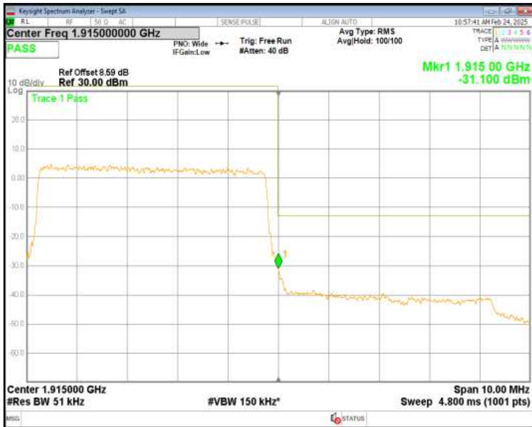
Band25 16QAM BW=5MHz Channel=26665 RB Size=25 Position=#0
