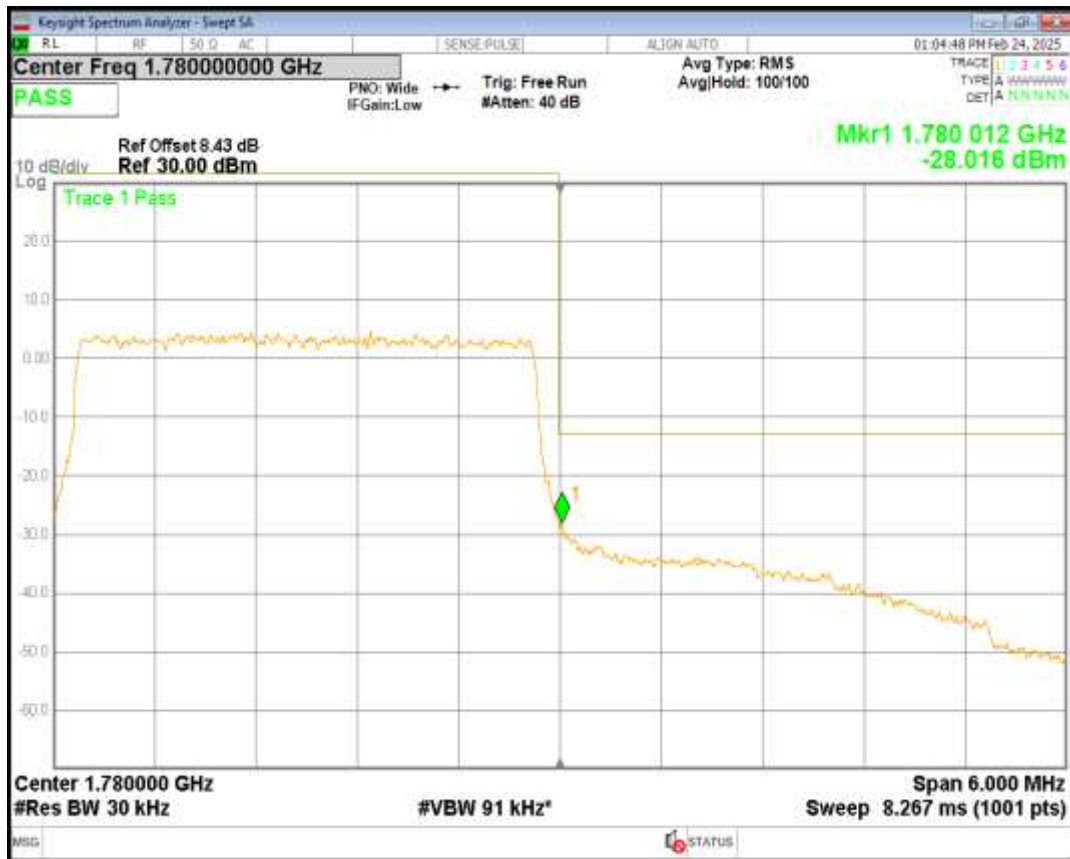
Band66 16QAM BW=3MHz Channel=132657 RB Size=15 Position=#0
