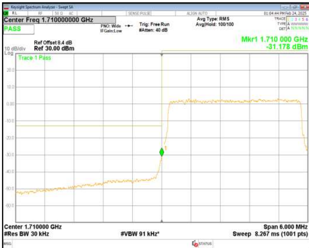
Band66 QPSK BW=3MHz Channel=132657 RB Size=15 Position=#0
