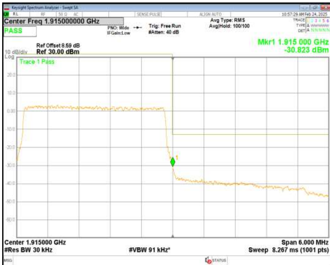
Band25 QPSK BW=5MHz Channel=26065 RB Size=25 Position=#0
