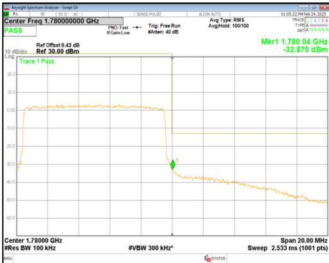
Band66 QPSK BW=15MHz Channel=132047 RB Size=75 Position=#0
