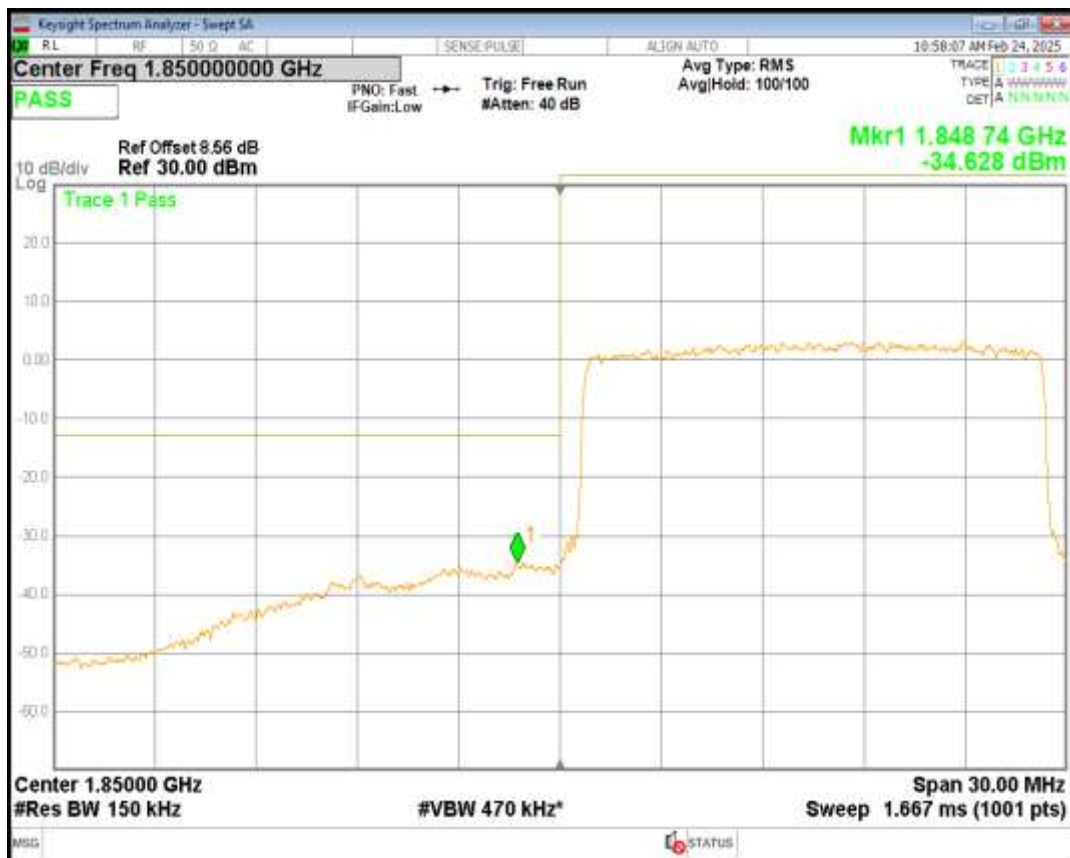
Band25 QPSK BW=15MHz Channel=26615 RB Size=75 Position=#0
