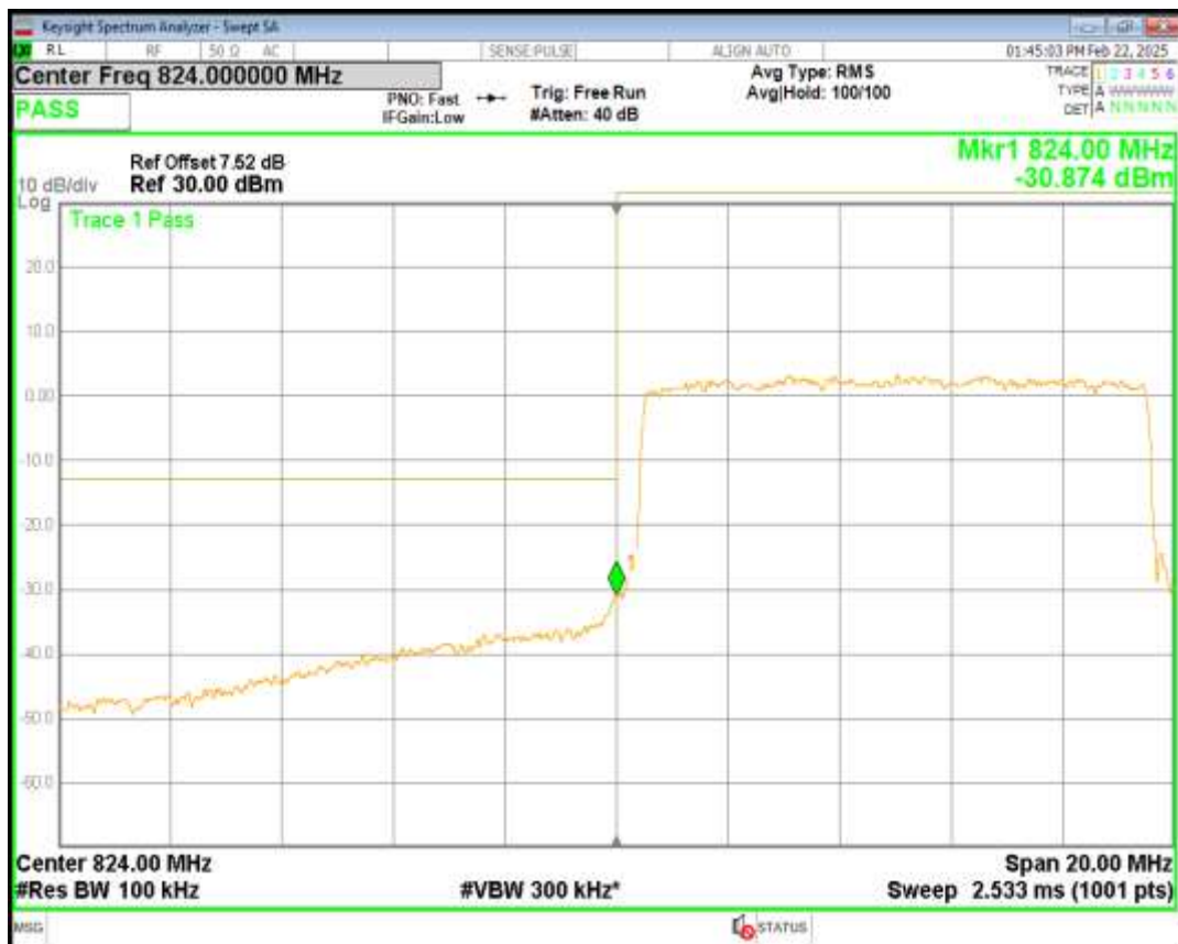
Band5 QPSK BW=10MHz Channel=20600 RB Size=50 Position=#0
