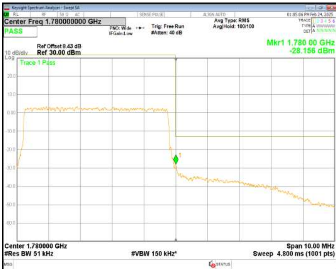
Band66 QPSK BW=10MHz Channel=132022 RB Size=50 Position=#0
