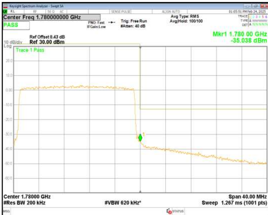
Band7 QPSK BW=5MHz Channel=20775 RB Size=25 Position=#0
