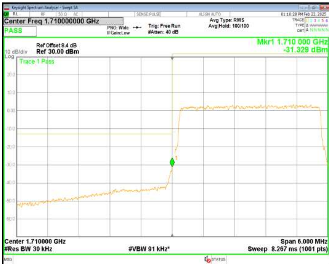
Band4 QPSK BW=3MHz Channel=20385 RB Size=15 Position=#0
