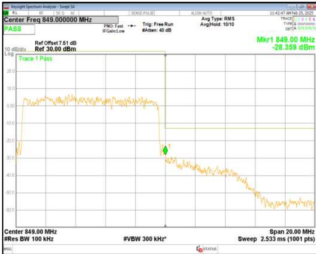
Band26(824-849) 16QAM BW=10MHz Channel=26990 RB Size=50 Position=#0
