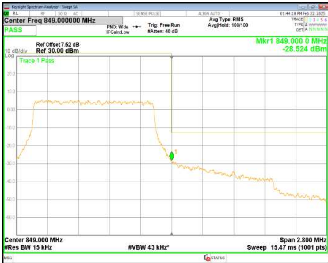
Band5 16QAM BW=1.4MHz Channel=20643 RB Size=6 Position=#0
