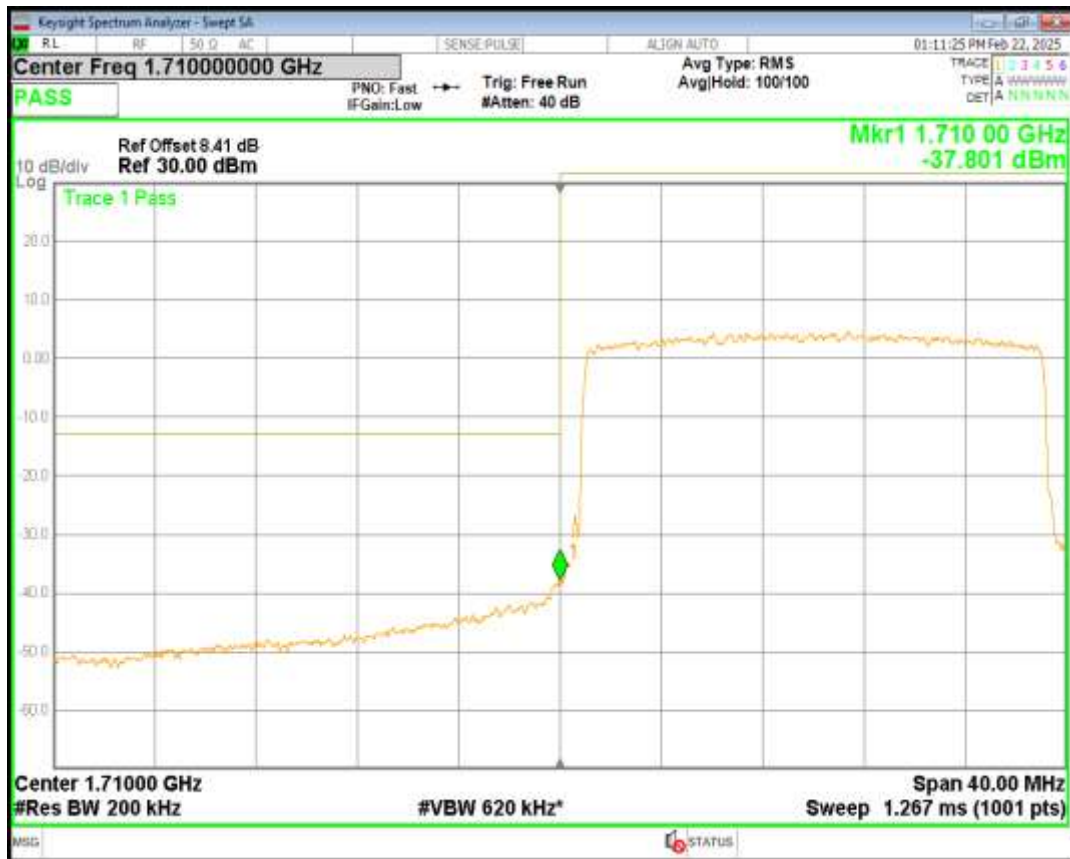
Band4 16QAM BW=20MHz Channel=20050 RB Size=100 Position=#0
