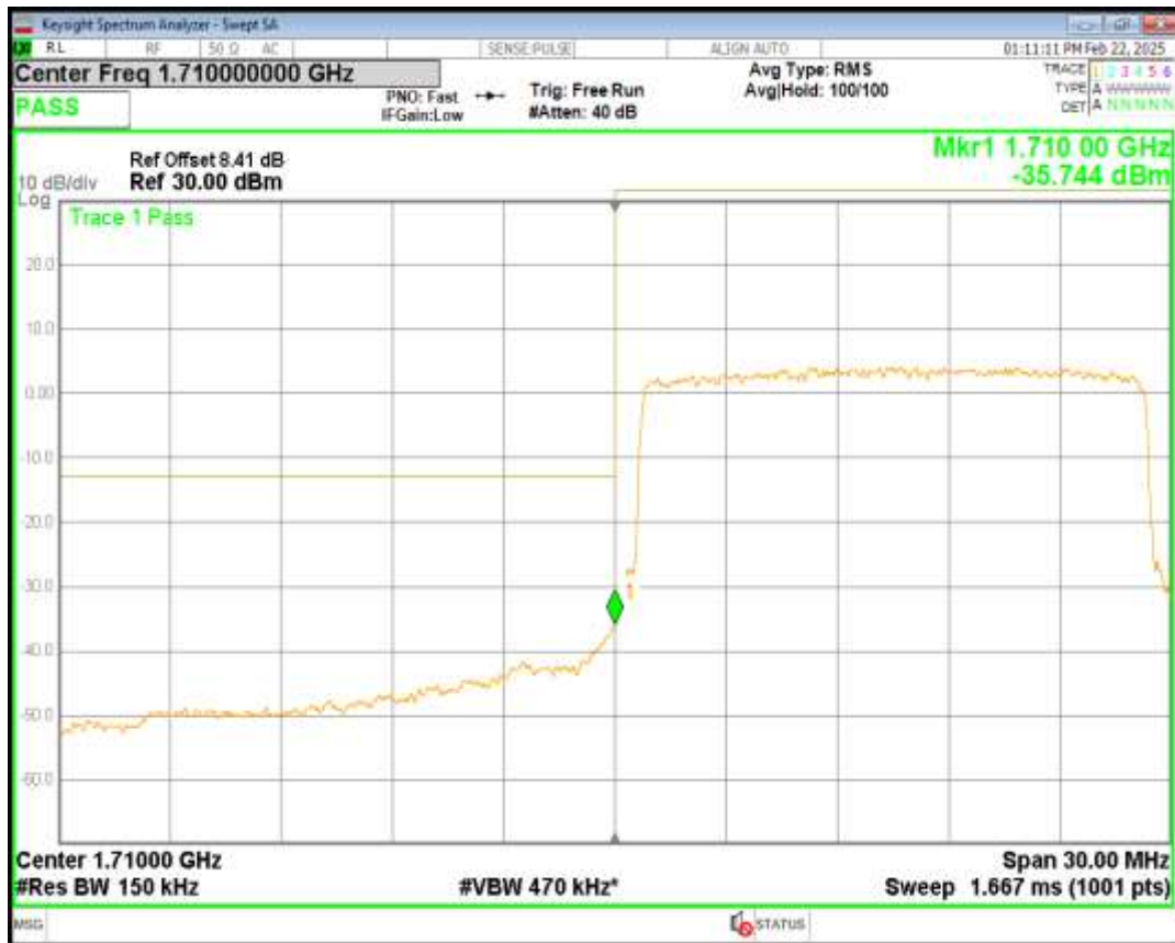
Band4 16QAM BW=15MHz Channel=20025 RB Size=75 Position=#0
