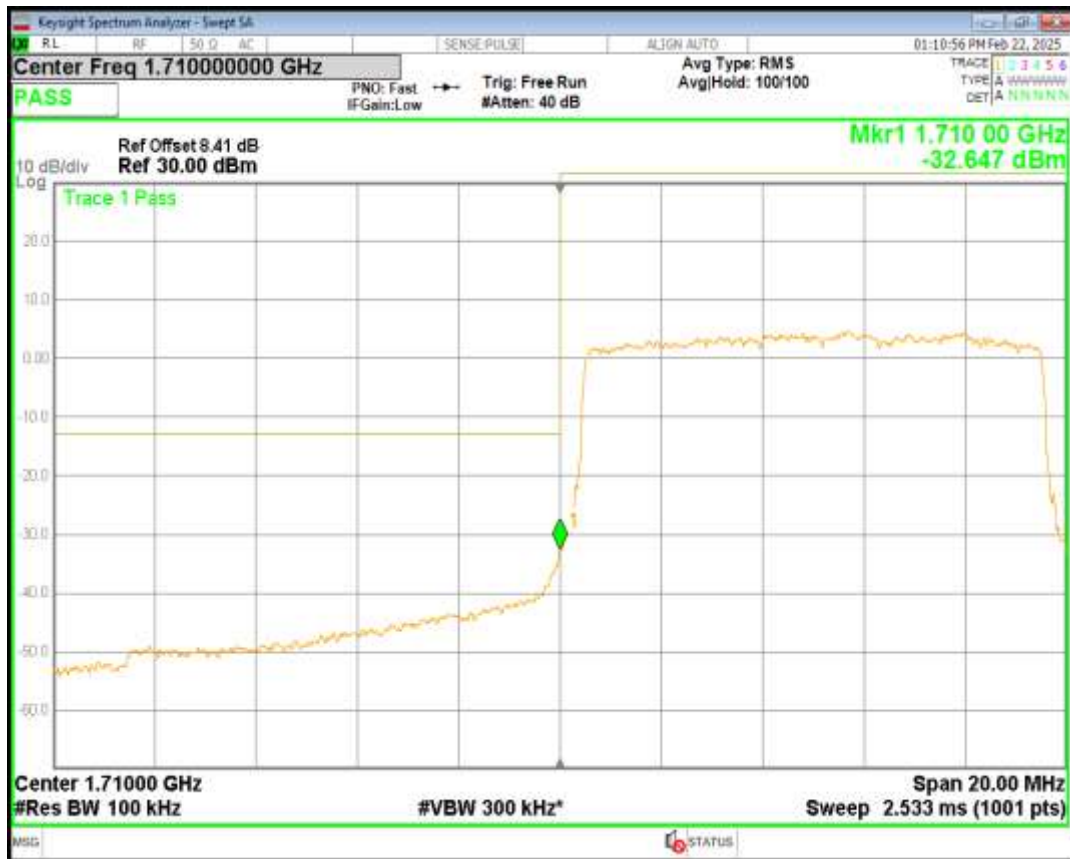
Band4 16QAM BW=10MHz Channel=20000 RB Size=50 Position=#0
