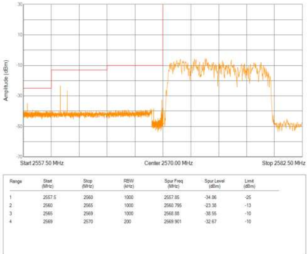
Band38 QPSK BW=10MHz Channel=38200 RB Size=50 Position=#0
