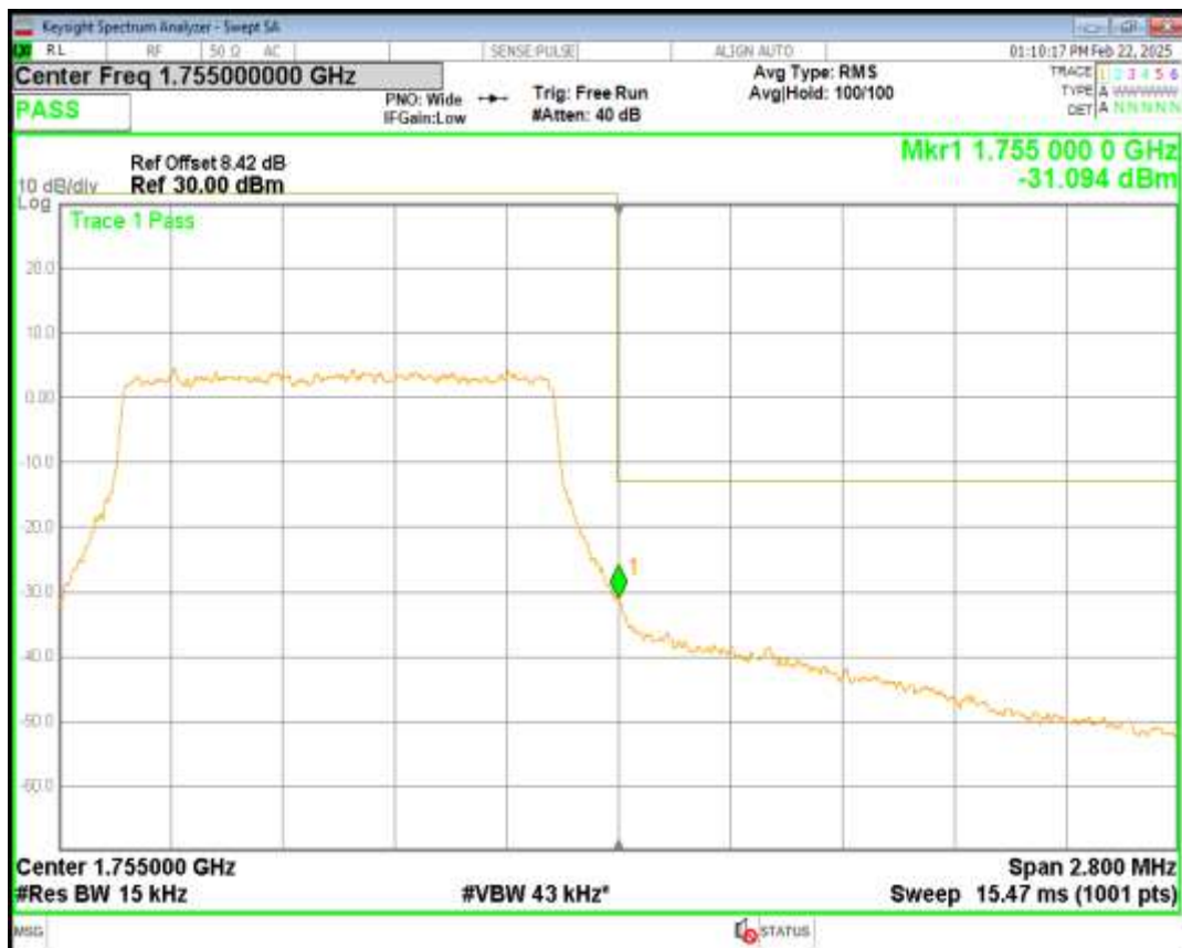
Band4 QPSK BW=3MHz Channel=19965 RB Size=15 Position=#0
