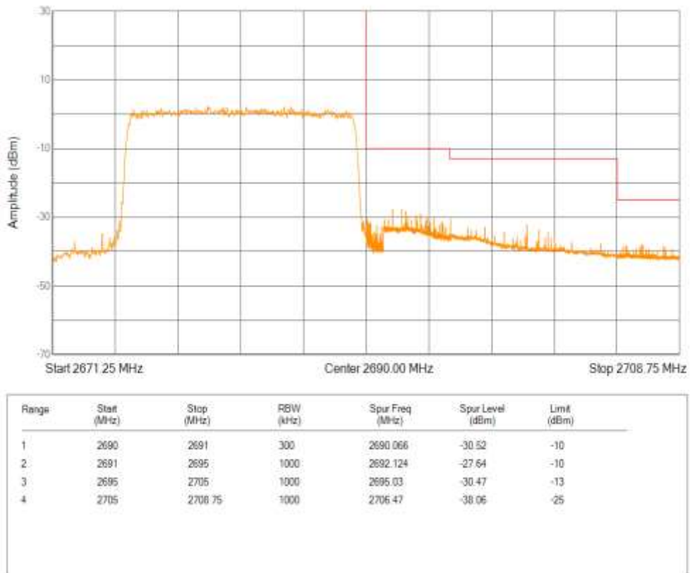
Band41 QPSK BW=20MHz Channel=39750 RB Size=100 Position=#0
