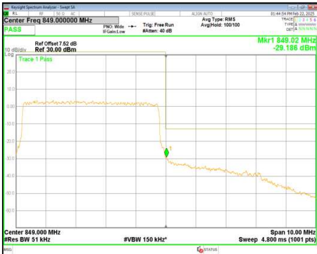
Band5 QPSK BW=10MHz Channel=20450 RB Size=50 Position=#0
