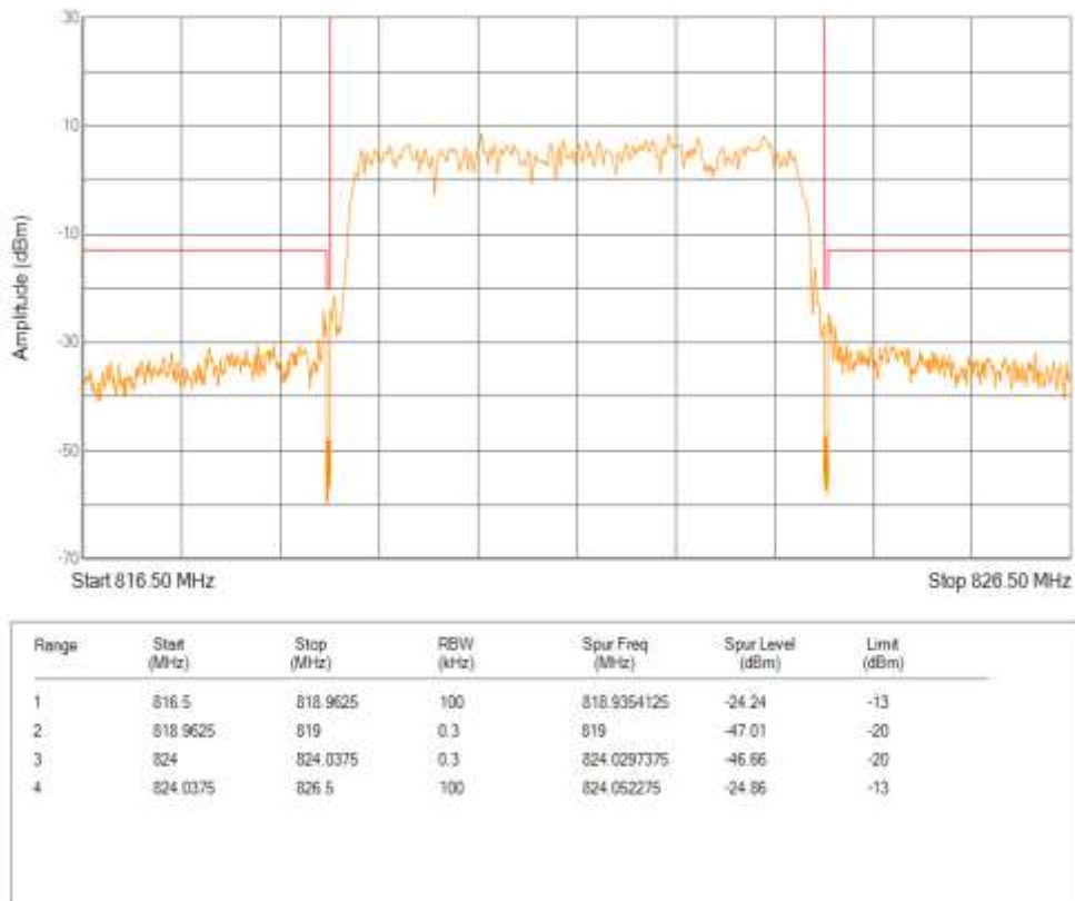
Band26(814-824) QPSK BW=10MHz Channel=26740 RB Size=50 Position=#0
