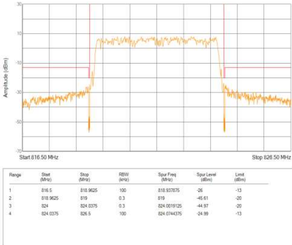
Band26(814-824) 16QAM BW=5MHz Channel=26765 RB Size=25 Position=#0
