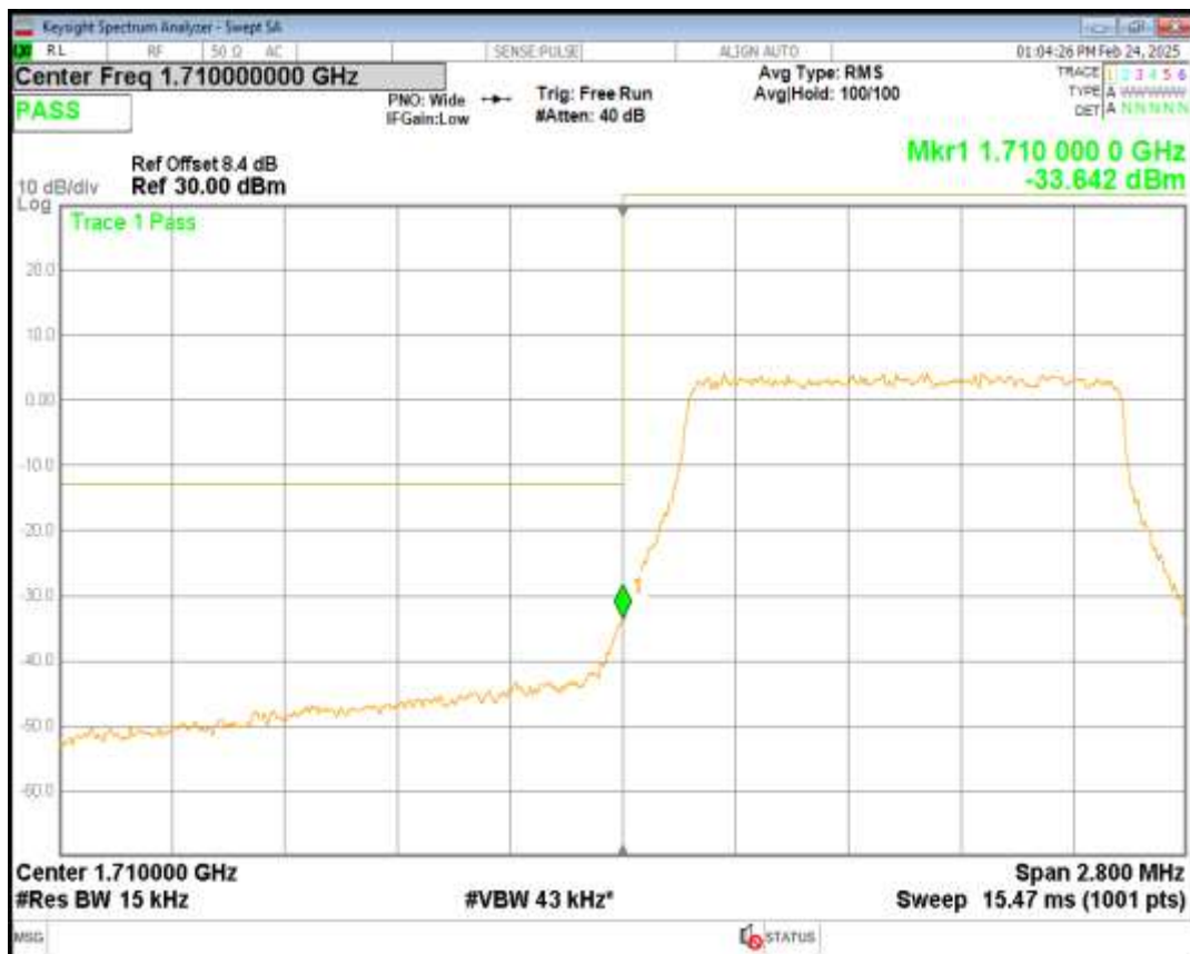
Band66 QPSK BW=1.4MHz Channel=132665 RB Size=6 Position=#0
