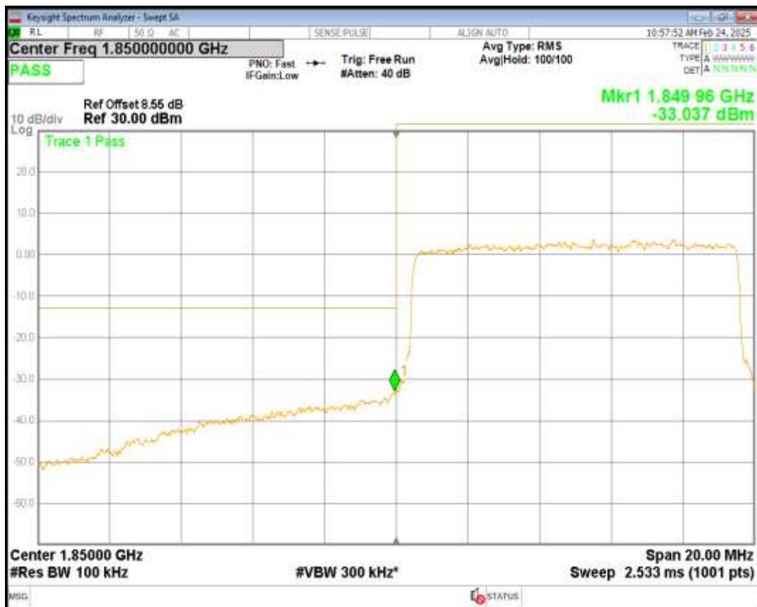
Band25 QPSK BW=10MHz Channel=26640 RB Size=50 Position=#0
