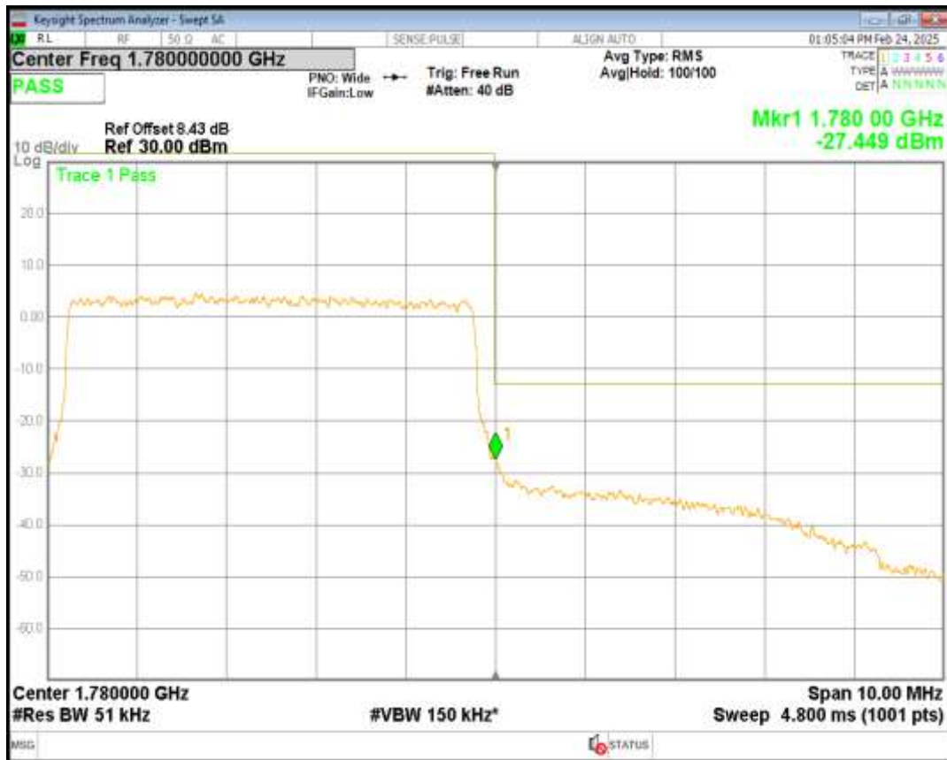
Band66 16QAM BW=5MHz Channel=132647 RB Size=25 Position=#0
