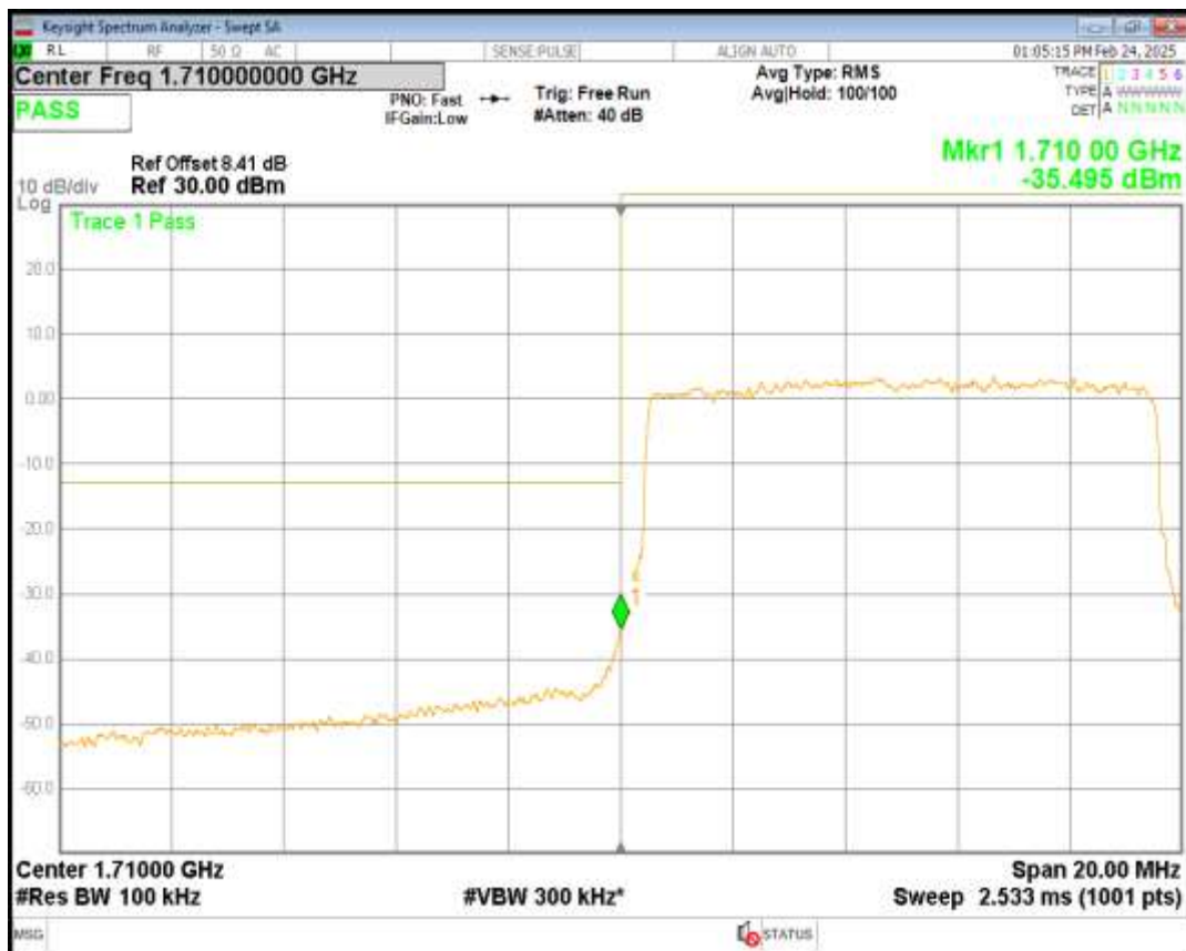
Band66 QPSK BW=10MHz Channel=132622 RB Size=50 Position=#0
