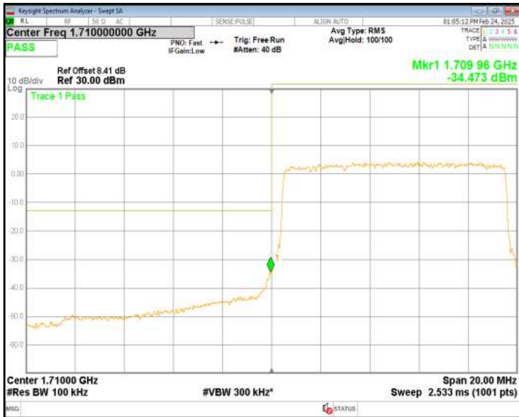
Band66 16QAM BW=10MHz Channel=132022 RB Size=50 Position=#0
