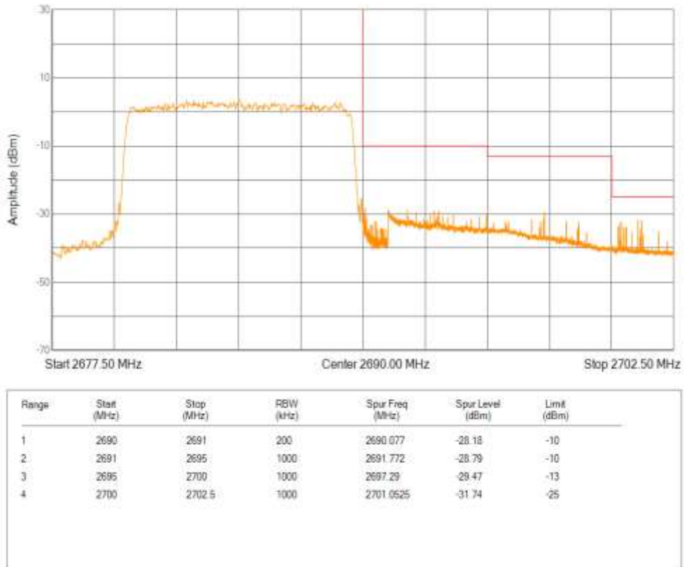
Band41 16QAM BW=10MHz Channel=41540 RB Size=50 Position=#0
