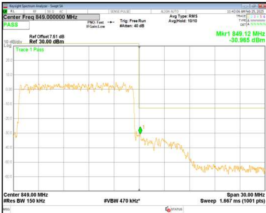
Band38 QPSK BW=15MHz Channel=38175 RB Size=75 Position=#0
