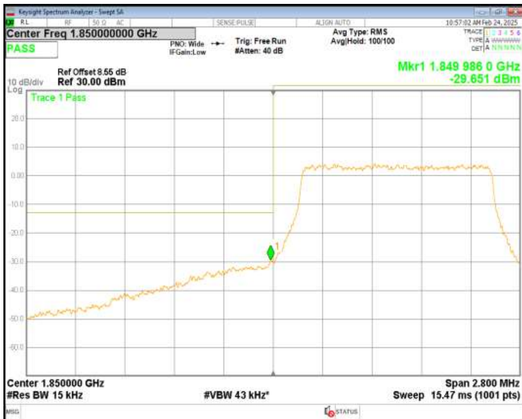
Band25 QPSK BW=1.4MHz Channel=26683 RB Size=6 Position=#0
