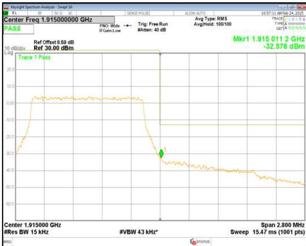
Band25 QPSK BW=3MHz Channel=26055 RB Size=15 Position=#0
