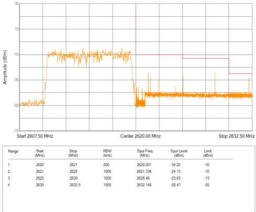
Band38 QPSK BW=15MHz Channel=37825 RB Size=75 Position=#0
