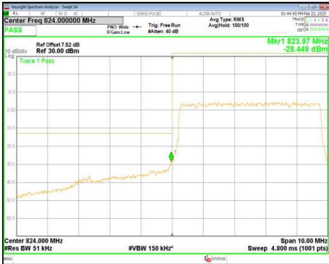
Band5 16QAM BW=5MHz Channel=20425 RB Size=25 Position=#0
