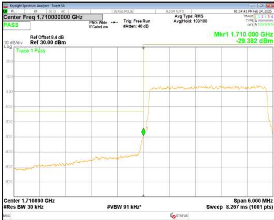
Band66 16QAM BW=3MHz Channel=131987 RB Size=15 Position=#0
