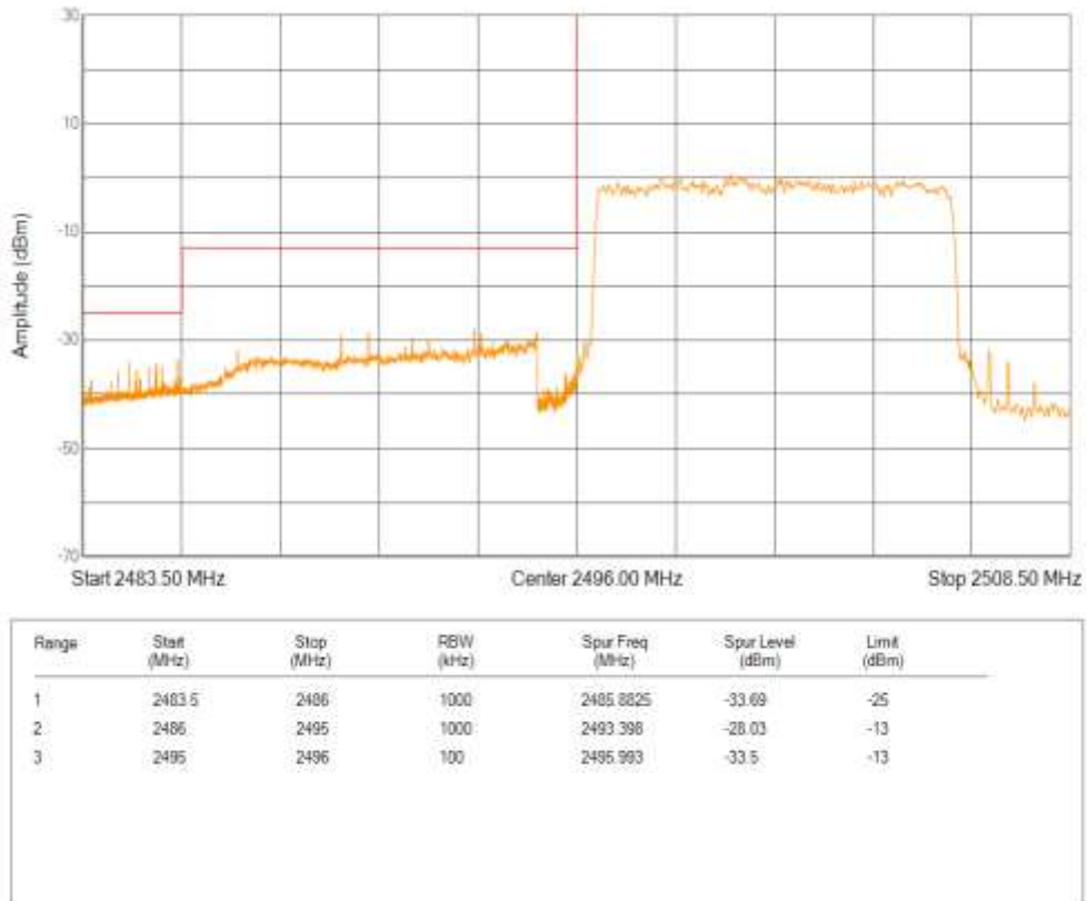
Band41 16QAM BW=10MHz Channel=39700 RB Size=50 Position=#0
