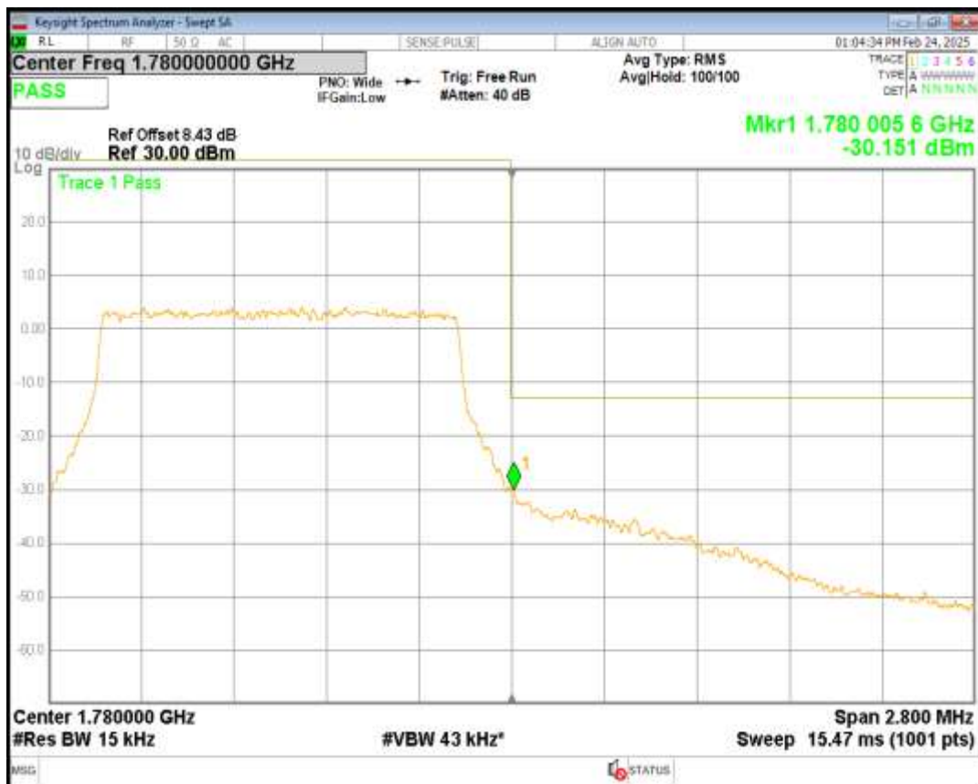
Band66 QPSK BW=3MHz Channel=131987 RB Size=15 Position=#0
