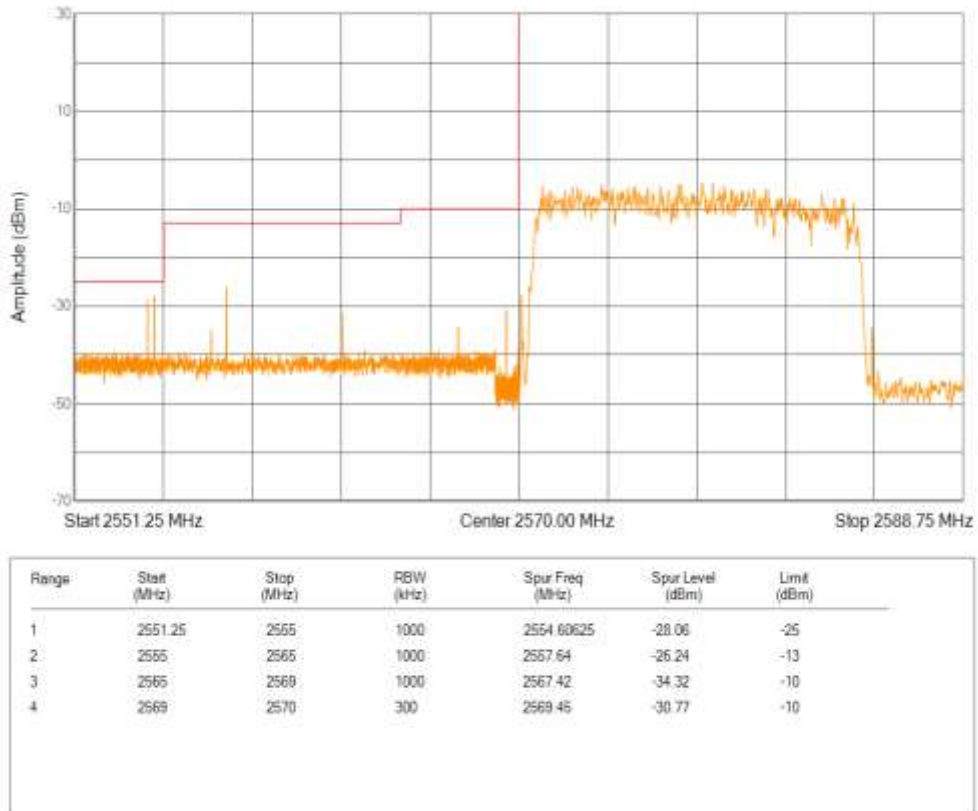
Band38 16QAM BW=15MHz Channel=38175 RB Size=75 Position=#0
