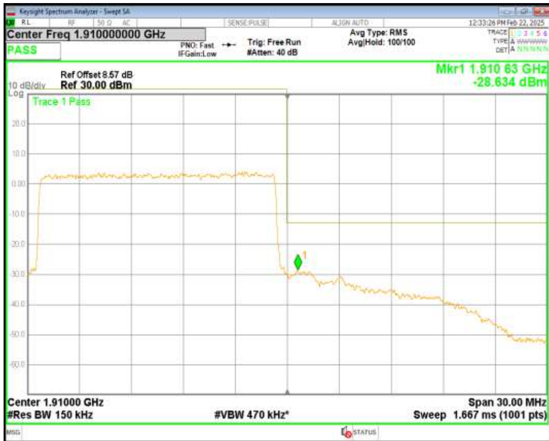
Band2 16QAM BW=15MHz Channel=19125 RB Size=75 Position=#0
