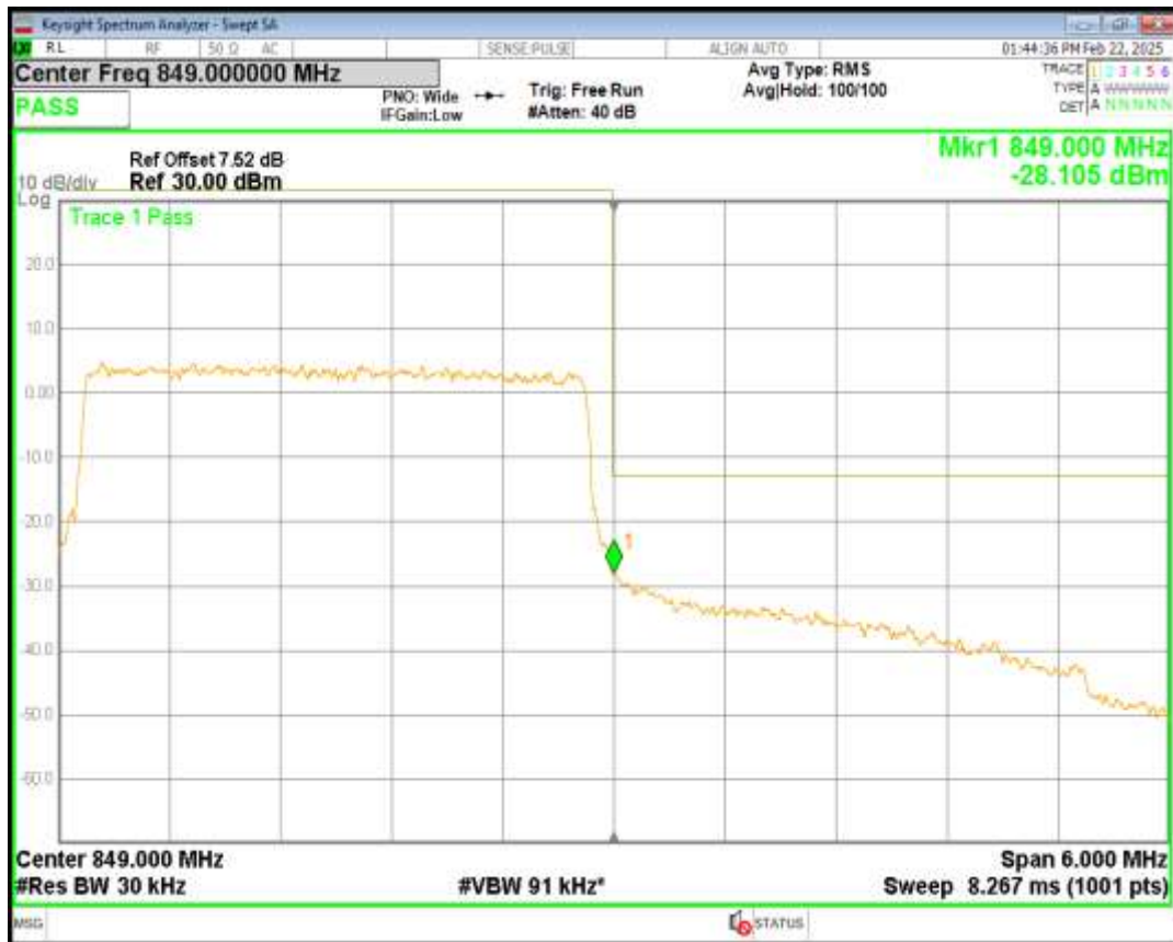
Band5 16QAM BW=3MHz Channel=20635 RB Size=15 Position=#0
