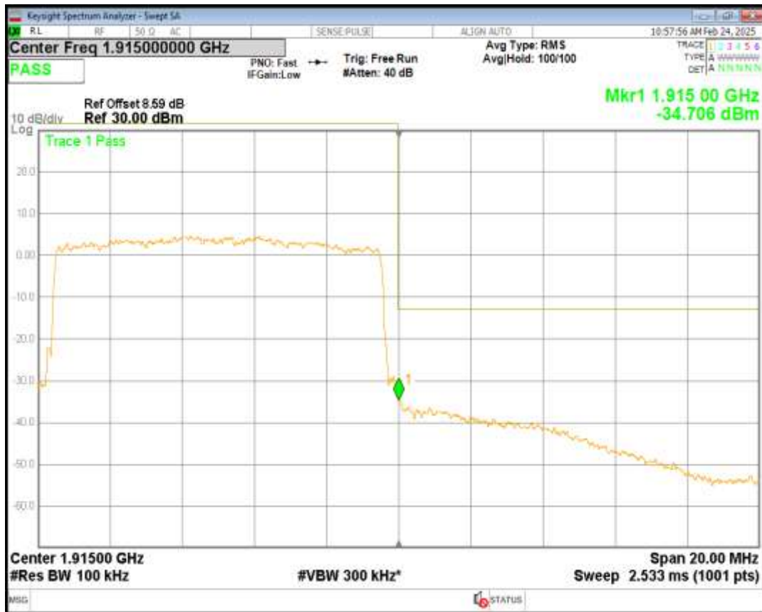
Band25 16QAM BW=10MHz Channel=26640 RB Size=50 Position=#0
