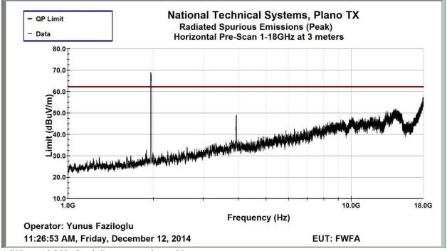
1GHz – 18GHz Peak Prescan at 3m – V
