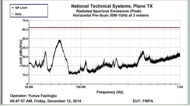
30MHz - 1GHz Peak Prescan at 3m - V
