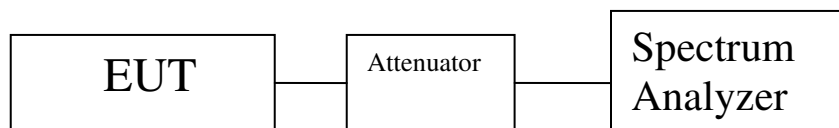
Figure 2. Block Diagram, Occupied Bandwidth Test Setup
