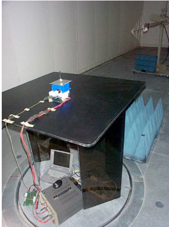
WaveNet BOOMER II tested for ERP 900 MHz band
