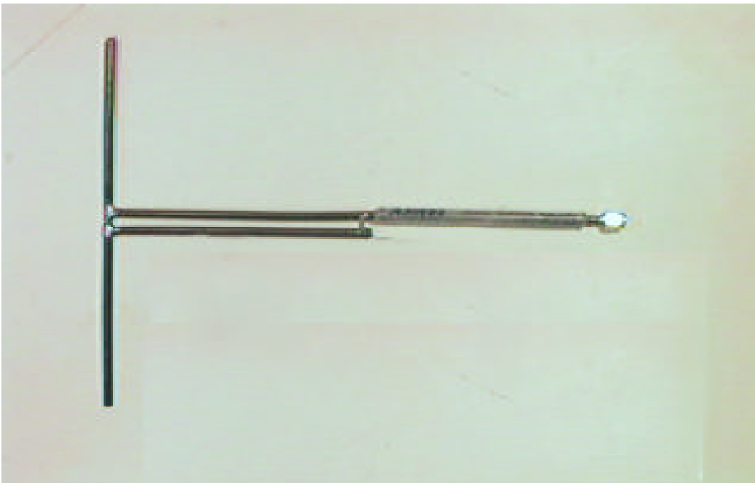
Reference Dipole Antenna Used for ERP Measurement
