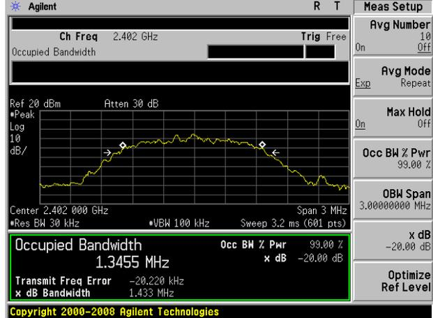
20dB Bandwidth plot on channel 39 (1Mbps)
