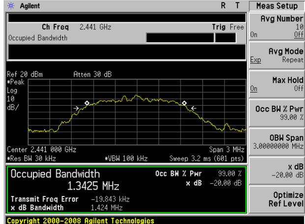
20dB Bandwidth plot on channel 78 (1Mbps)
