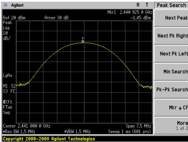
Peak output Power plot on channel 78 (3Mbps)
