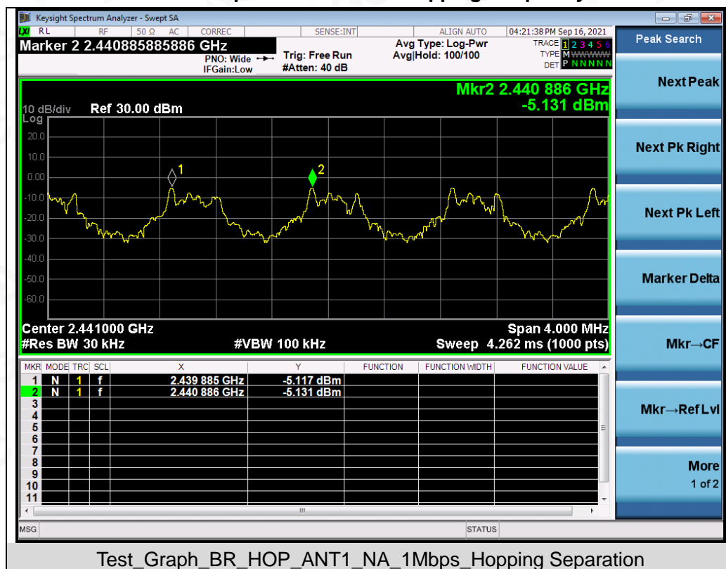
Test Graphs of Number of Hopping Frequency
