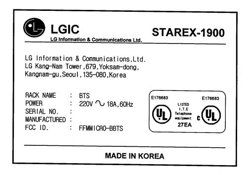
name plate of this type, or one similar to it, will be affixed to every base station. This label is permanent, indeliable, and tamper evident.
