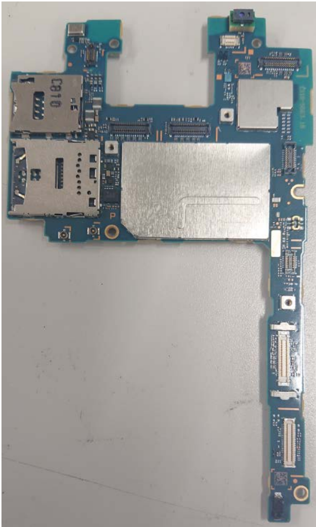
Internal Main PWB with Shield cases (Front-side)
