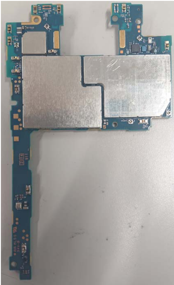
Internal PWB with Shield cases (Rear-side)
