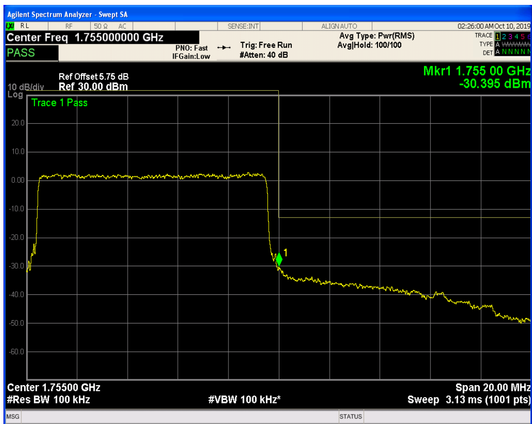
LTE Band4 QPSK BW=15MHz Channel=20025 RB Size=1 Position=#0
