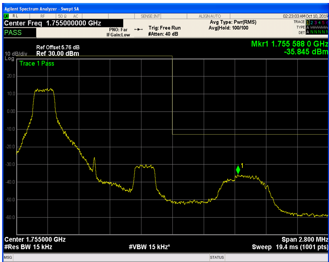
LTE Band4 QPSK BW=1.4MHz Channel=20393 RB Size=6 Position=#0
