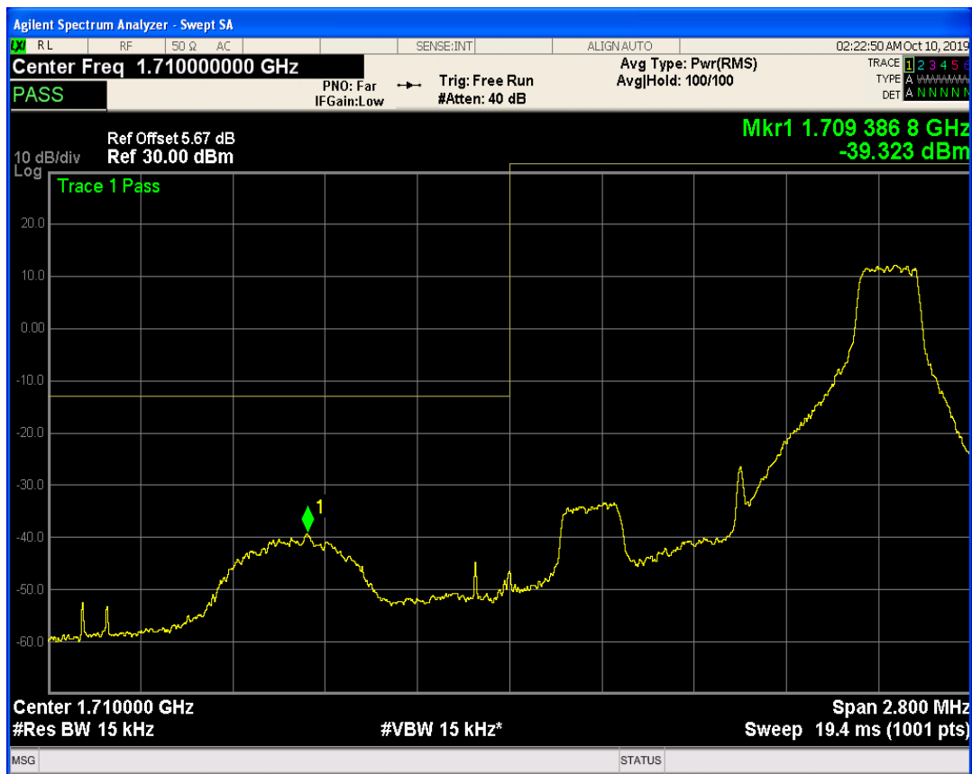
LTE Band4 QAM16 BW=1.4MHz Channel=19957 RB Size=6 Position=#0
