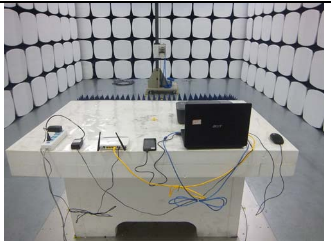
Radiated Spurious Emissions Test Setup Above 1GHz
