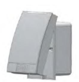
Once the screw is removed pull the reader out and up to remove it from the wall mount bracket.
