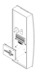
Position the SABRE module (with logo up), 5 onto the Hiroshi connector and press firmly to make a connection.
